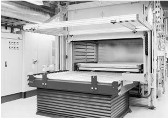
14.13 Medium wave IR oven for the curing of carbon composites. (Source: Voetsch.)
