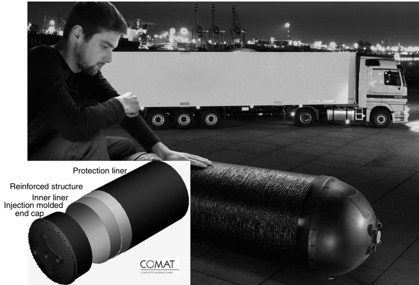
7.12 Air pressure vessels for truck application manufactured using direct impregnation technique. (Courtesy of COMAT Composite Materials GmbH, Germany.)
