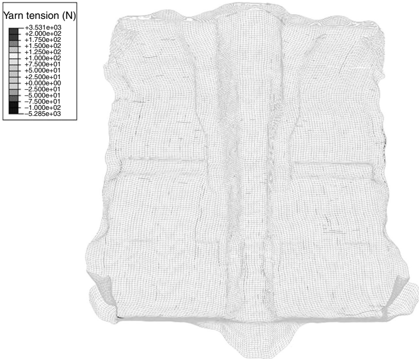
6.45 Yarn tension contour for the 90/0 fabric orientation.
