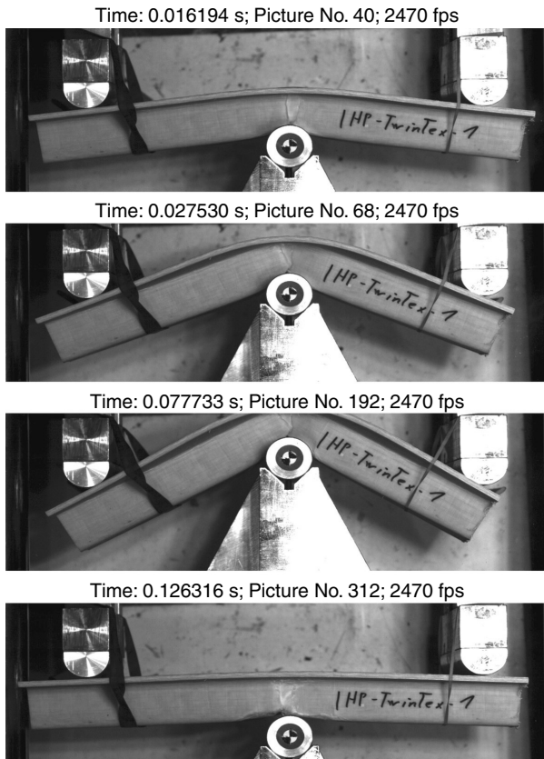
8.33 Crash test behavior of a closed cap profile (IVW GmbH). (From reference 37.)
