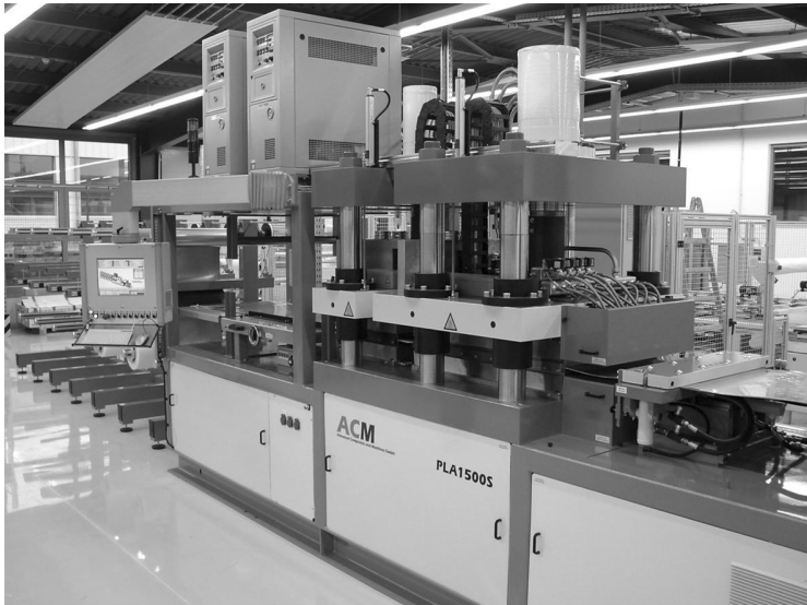
8.18 Continuous compression molding (CCM) machine (IVW GmbH). (From reference 37.)
