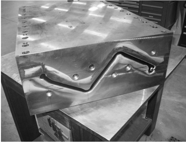
8.7 Pultrusion die (manufactured by MPI-Ft. Worth Texas). (From reference 19.)
