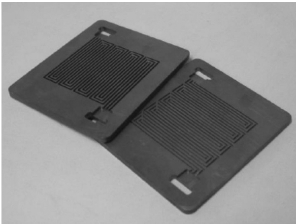
3.5 Compression molded polymer-graphite bipolar plates for direct methanol fuel cell (Chen et al. , 2010).
