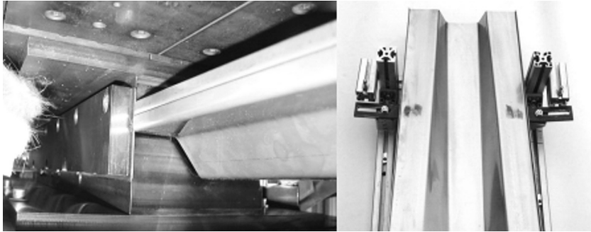
8.27 Pre-forming unit located in front of the CCM machine (xperion Aerospace GmbH). (From reference 38.)
