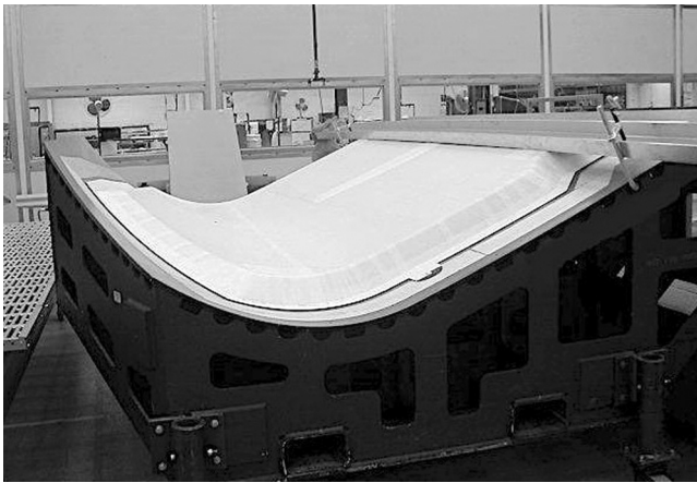
13.11 Cured test article placed on process tooling to measure dimensional fidelity.
