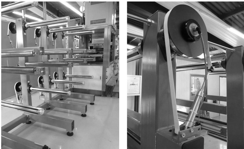
8.21 Creel of the CCM press (left picture) and strap brake (right picture) (IVW GmbH). (From reference 37.)
