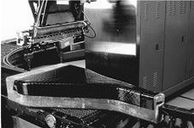
14.22 E-beam cured composite laminate. (From reference 27.)
