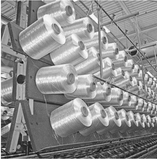
8.5 Creel assembled with glass fiber (TEXMER GmbH&Co. KG). (From reference 18.)
