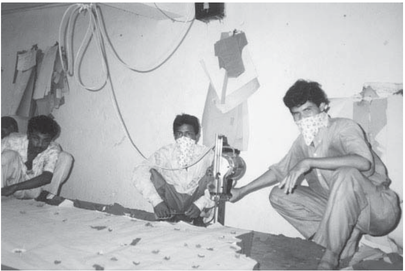
Figure 10. Men use jigsaws to cut cloth from patterns, Dhaka. They wear cloths over their noses and mouths to protect their lungs from the fibers and dust that permeate the factory.
