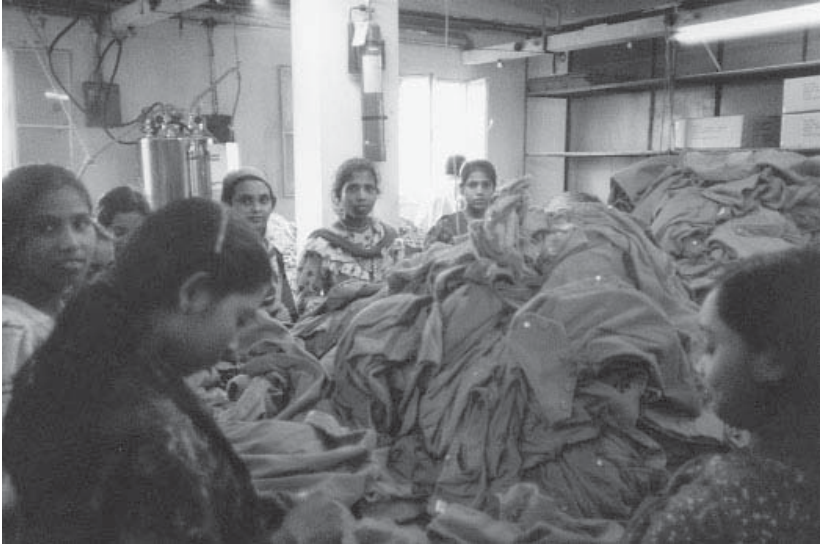
Figure 7. Helpers, mostly young women who are apprentice sewing-machine operators, trim excess thread from finished clothes in a garment factory, Dhaka.
