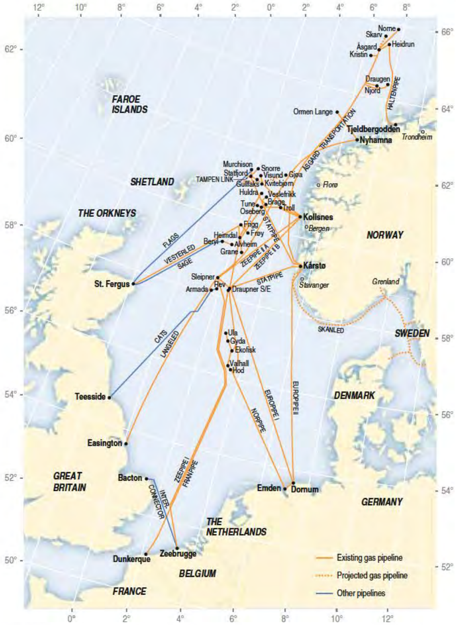
Fig. 11.1 The transport network on the Norwegian Continental Shelf (Ministry of Petroleum and Energy/Norwegian Petroleum Directorate 2009)
