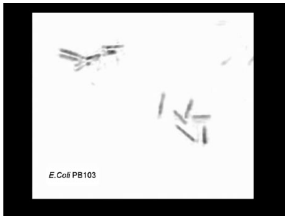
Fig. 1.14 E.coli bacteria imaged with a blue laser. Pinhole–object distance 300 \mu\text{m} , pinhole–screen distance 15 mm, pinhole 0.5 \mu\text{m} . Bacteria diameter about 1 \mu\text{m}
