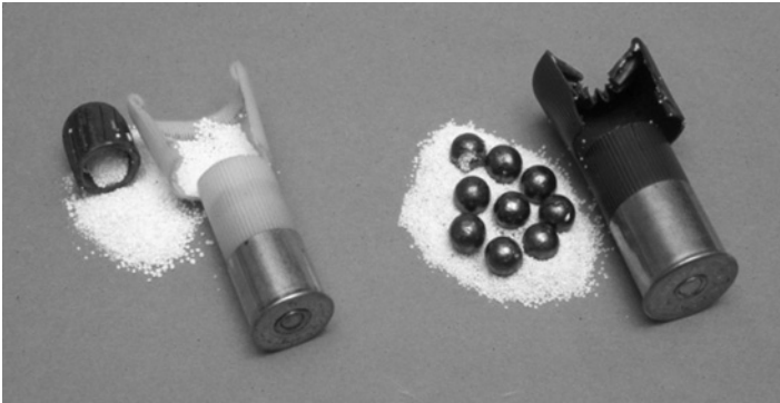
Fig. 12. Buffered shot shell loads (l. slug, r. buckshot)
