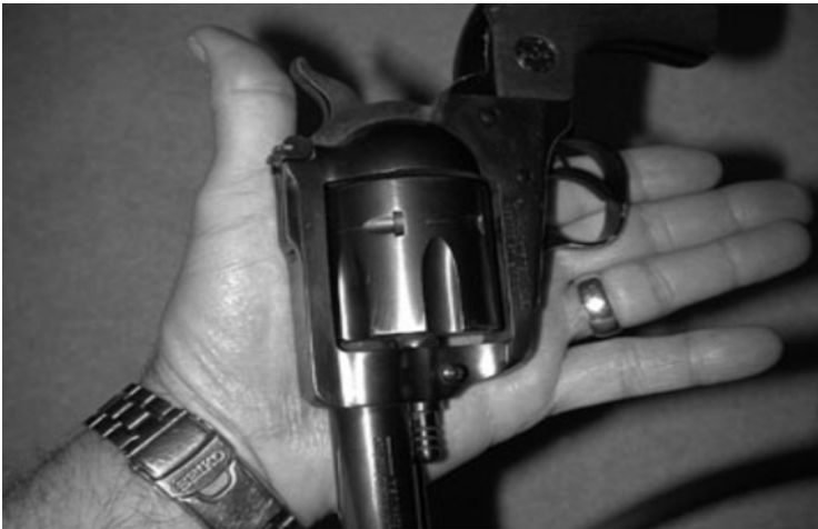
Fig. 18. Left-hand orientation based on cylinder gap deposit on palm.
