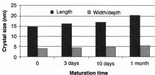
Figure 2.4 Variation of nanocrystalline apatite dimensions with maturation time. Reprinted from Ref. [235] with permission.
