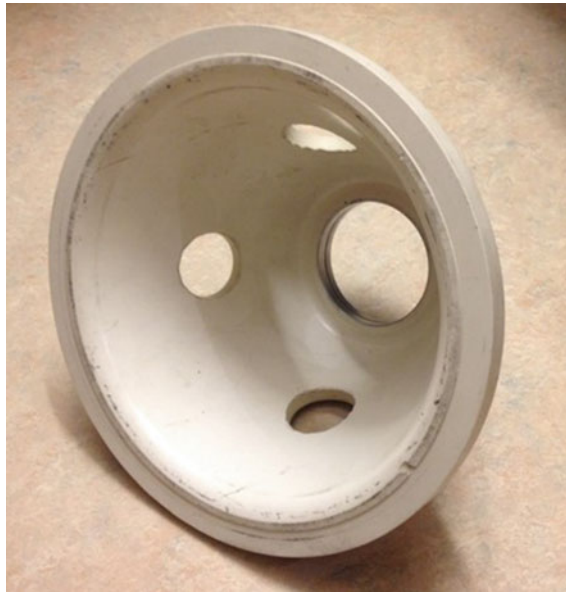
Fig. 4.7 Epoxy insulator with a metal conductor and ring contact in the centre
