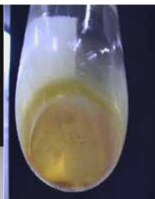
Colour good Transparency good Sediment poor
