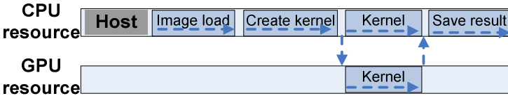
Fig. 4. Proposed parallel processing of photomosaic using both GPU and CPU
