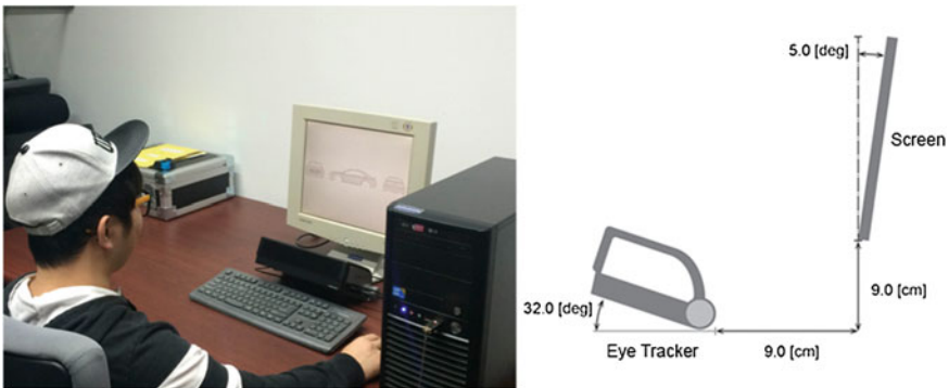
Fig. 12.3 Image of eye tracking experimentation setting taken from Hyun et al. [11]
