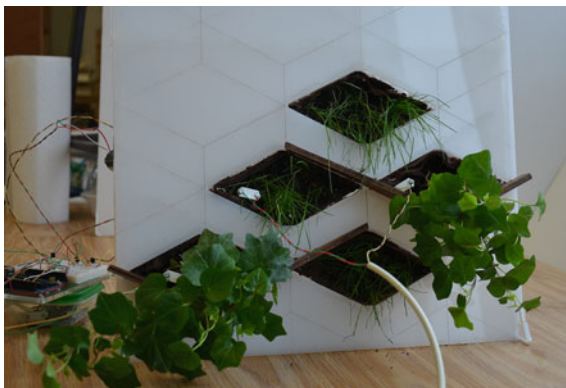
Fig. 18.11 The self-watering green wall installation
