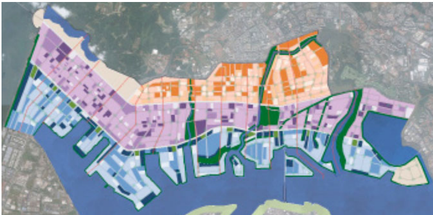
Fig. 10.3 Ecotopia: land use master plan. The site is divided into three different mixed-use belts, from top to bottom mainly residential, mainly industrial and mainly commercial. Credits Andrea Meinarti Rachmat, Tey Hui Ping Serene, Delon Leonard, Wu Xin Peng, Loh Sze Sian (tutor: Oscar Carracedo)
