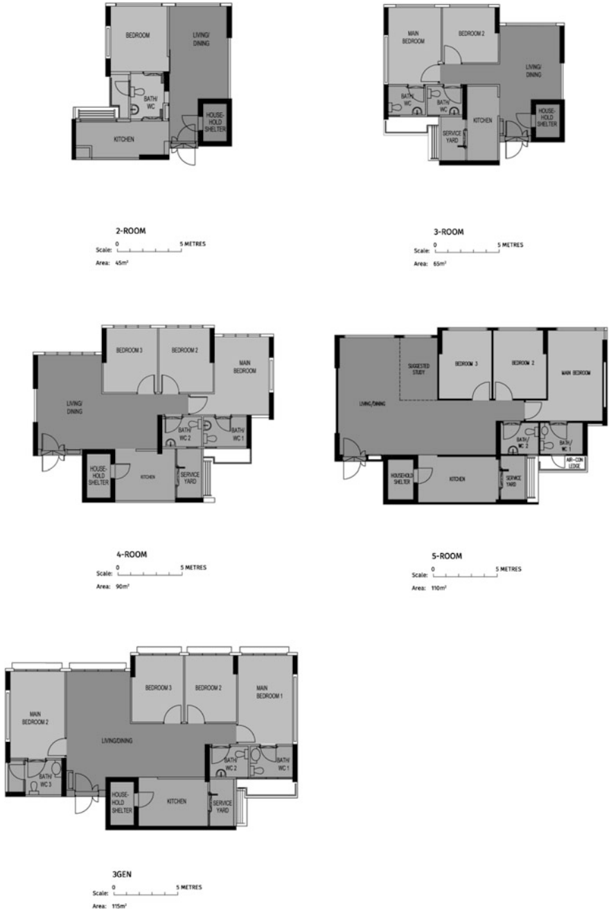
Fig. 1.1 HDB floor plans of various flat typologies. Source Housing Development Board (2015), pp. 18–22
