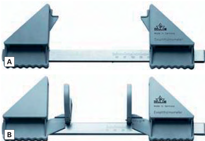
Fig. 84.1 Types of exophthalmometer. Hertel (A); Naugle (B). Note that the Naugle instrument rests on the forehead and cheek, whereas the Hertel rests in the lateral canthus.
