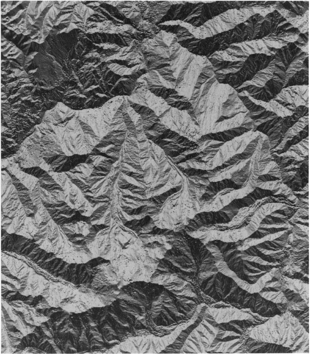
Fig. 11. Slope aspect image of the Nanga Parbat massif showing slope orientation in a north–south direction ( \cos \phi_T ). The image clearly depicts the first-order topography and the orientation of the massif in a northeasterly direction. The massifs are highlighted by north-facing slopes resulting from the influence of the Indus River. Third-order topography is also highlighted in many basins on the north side of Nanga Parbat.
