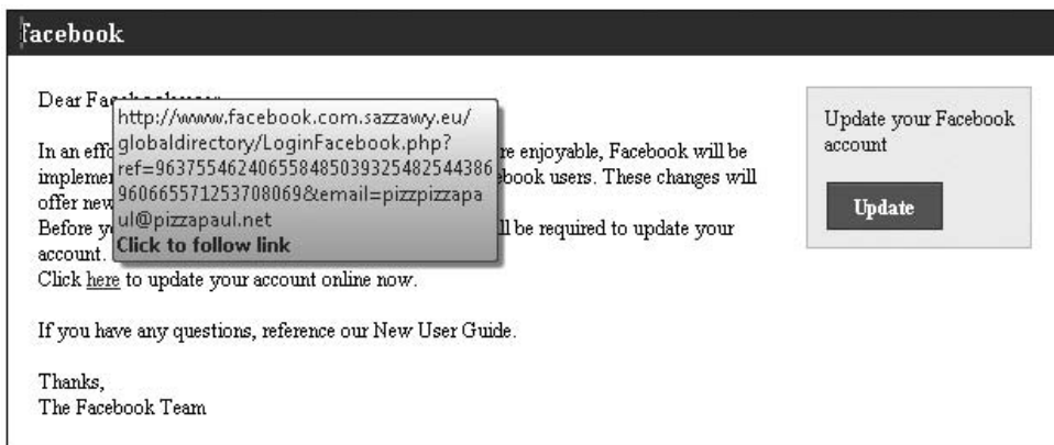
Figure 15.2 View the Web address to which a link in an e-mail points.
