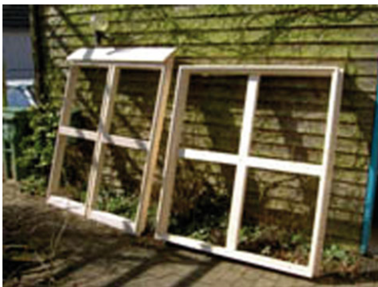
Figure B.12 Prototype window scale 1:1 made of pine wood, without the glass panes, showing the outer and inner window component separately.
