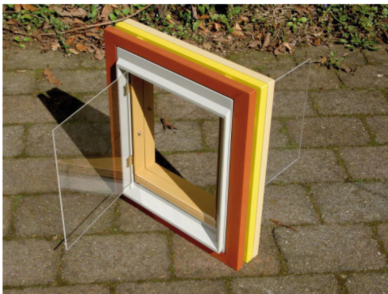
Figure B.11 Model scale 1:10 of the window in a cavity wall.
