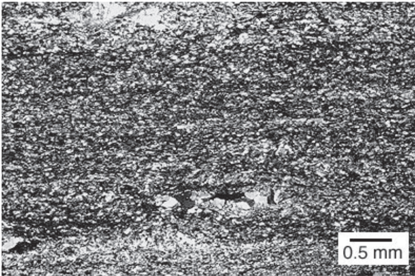
FIGURE 3.21 Ascribing meaning to the shape of a natural object: the shape and orientation of the mineral grain in this photomicrograph are interpreted as evidence that the rock has undergone shearing. SOURCE: The University of North Carolina, Chapel Hill, Department of Geological Sciences.
