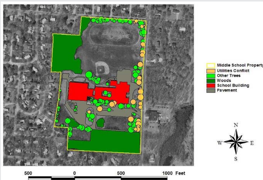
FIGURE 8.5 Trees conflicting with utility lines.
