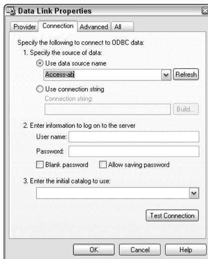
**Figure 20-3:** Use the Data Link Properties dialog box to configure your data source within AutoCAD.
