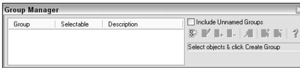
**Figure 10-46:** Use the Group Manager window to create and manage groups in AutoCAD LT.
