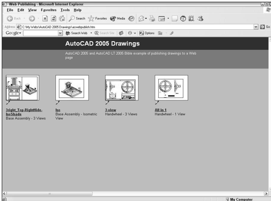
**Figure 28-11:** A preview of some drawings using the Array of Thumbnails template and DWF files. You can click on any thumbnail to see the full-size DWF file. Note the i-drop icons.
