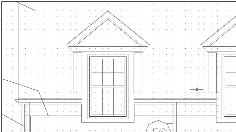
**Figure 4-16:** A portion of a drawing with the grid turned on and set to 6 inches.
