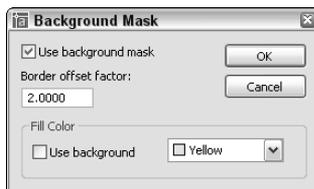
**Figure 13-19:** Use the Background Mask dialog box to create a background around your text so that no other object obscures the text.
