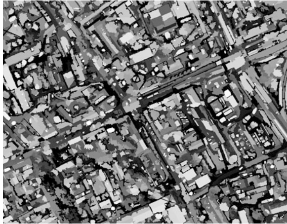
Fig. 14 Segmentation by ellipticity (black or “ying”: more elongated, white or “yang” is round) Urban object extraction from heterogenous data sources (produced by the authors using Bentley Microstation based Terrasolid engineering planning environment and Trimble eCognition image analysis toolsets)
