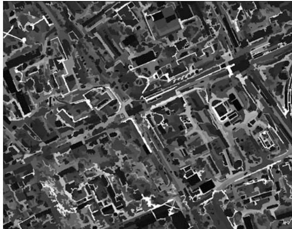
Fig. 15 Segmentation by compactness. Urban object extraction from heterogenous data sources (produced by the authors using Bentley Microstation based Terrasolid engineering planning environment and Trimble eCognition image analysis toolsets)
