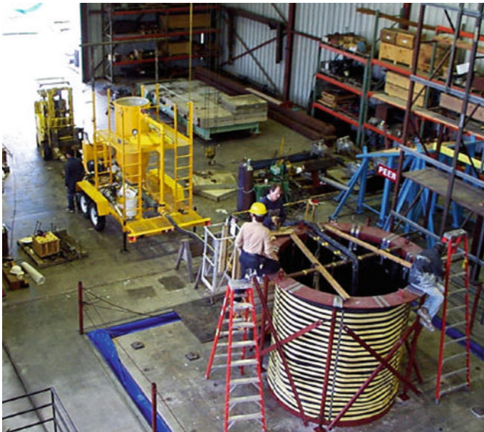
Fig. 6.30 Full-scale cylinder soil container mounted on a shaking table, with support struts, and soil mixer/pump in background (courtesy of Pacific Earthquake Engineering Research Center and PJ Meymand, University of California, Berkeley, and California Department of Transportation)
