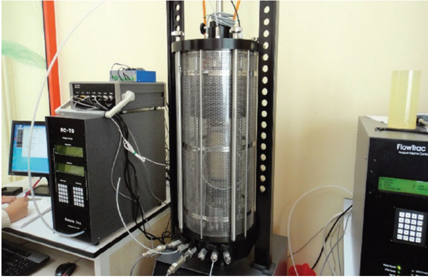
Fig. 6.24 Test apparatus for resonant column test (courtesy of Geocomp/GeoTesting Express)
