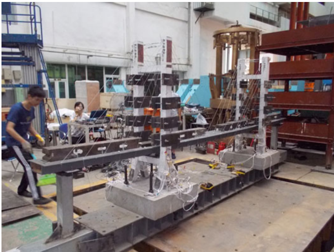
Fig. 6.28 Shaking table test for a cable-stayed bridge model on a 3 \times 3 m shaking table
