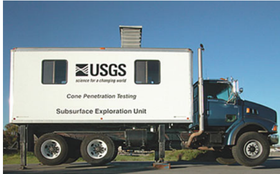
Fig. 1.21 A truck operating CPT (courtesy of USGS)
