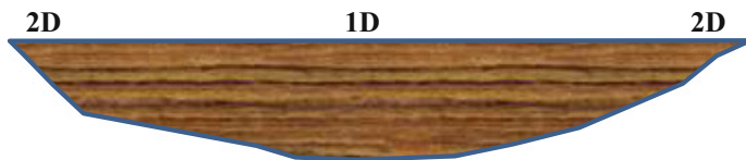
Fig. 3.35 A wide, shallow basin may allow for one-dimensional site-response analysis in the basin center but requires two-dimensional analysis for areas near edges
