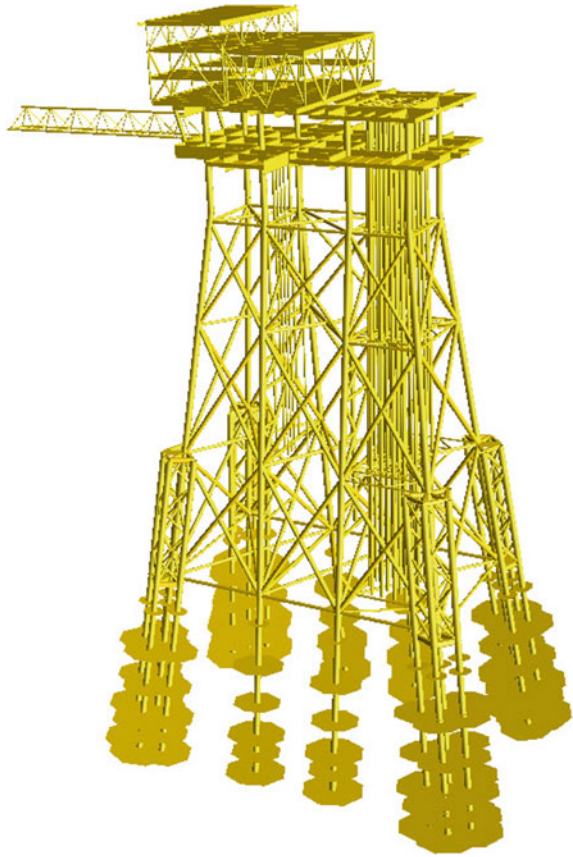
Fig. 21.9 Illustration of a pile foundation layout for a drilling platform as shown in Fig. 21.10 (disks attached to the pile foundations represent various soil layers)
