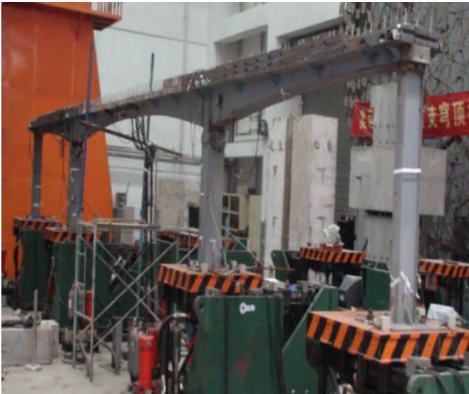
Fig. 6.29 Nine subarray shaking table system for scale-model test of large-scale prototype infrastructures (courtesy of Beijing Laboratory of Earthquake Engineering and Structural Retrofit, Beijing University of Technology)
