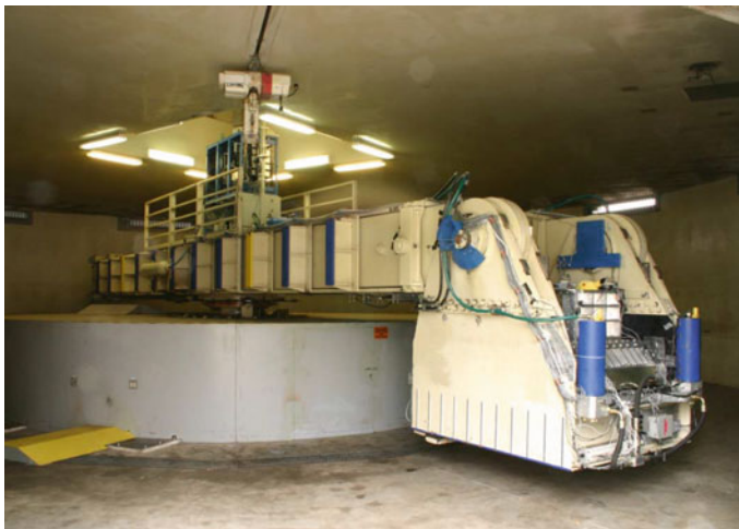
Fig. 6.32 Illustration of a typical centrifuge test [387]
