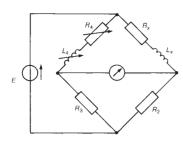
**Figure 27.2** Simple Maxwell bridge
