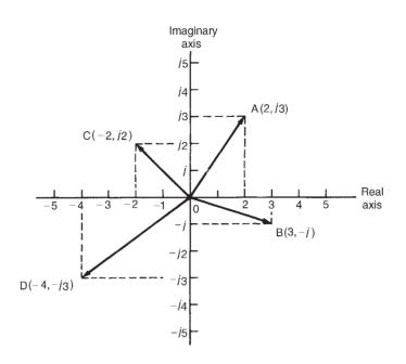
Figure 23.1 The Argand diagram
