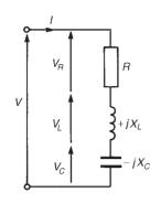
**Figure 28.1** R - L - C series *circuit*
