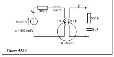
(a) Self impedance of primary circuit,  $Z_1 = 300 + j(500)(0.2 + 0.5)$ i.e.,  $Z_1 = (300 + j350)\Omega$
