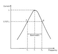
**Figure 28.6** Bandwidth and half-power points  $f_1$  and  $f_2$
