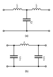
shown in Figure 42.13(b). The shunt element C in Figure 42.12(a) may be regarded as two capacitors in parallel, each of value C/2 as shown in the part of the ladder redrawn in Figure 42.12(b). (Note that for parallel capacitors, the total capacitance  $C_T$  is given by
