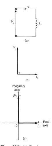
**Figure 24.2** (a) Circuit diagram (b) Phasor diagram (c) Argand diagram
