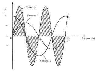
Figure 26.2 Power in a purely inductive a.c. circuit
