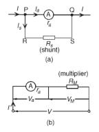
An **ammeter**, which measures current, has a low resistance (ideally zero) and must be connected in series with the circuit.
