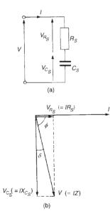
**Figure 39.2** (a) Circuit diagram (b) Phasor diagram
