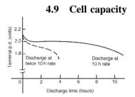
The **capacity** of a cell is measured in ampere-hours (Ah). A fully charged 50 Ah battery rated for 10 h discharge can be discharged at a steady current of 5 A for 10 h, but if the load current is increased to 10 A then the battery is discharged in 3-4 h, since the higher the discharge current, the lower is the effective capacity of the battery. Typical discharge characteristics for a lead-acid cell are shown in Figure 4.8.
