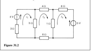
The mesh currents  $I_1$ ,  $I_2$  and  $I_3$  are shown in Figure 31.2. Using Kirchhoff's voltage law:
