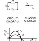
CURRENT AND VOLTAGE WAVEFORMS
