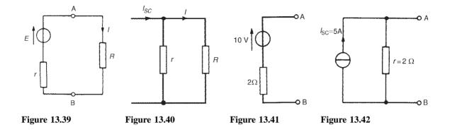
From Figure 13.40 it can be seen that, when viewed from the load, the source appears as a source of current  $I_{SC}$  which is divided between r and R connected in parallel.
