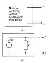
Figure 33.39 The Norton equivalent circuit
