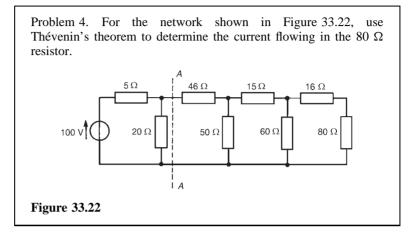
One method of analysing a multi-branch network as shown in Figure 33.22 is to use Thévenin's theorem on one part of the network at a time. For example, the part of the circuit to the left of AA may be reduced to a Thévenin equivalent circuit.
