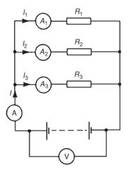
Figure 5.9 shows three resistors,  $R_1$ ,  $R_2$  and  $R_3$  connected across each other, i.e., in parallel, across a battery source of V volts.
