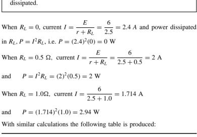
Problem 20. The circuit diagram of Figure 13.48 shows dry cells of source e.m.f. 6 V, and internal resistance 2.5 $\Omega$ . If the load resistance  $R_L$  is varied from 0 to 5  $\Omega$  in 0.5  $\Omega$  steps, calculate the power dissipated by the load in each case. Plot a graph of  $R_L$  (horizon-
