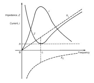
**Figure 28.4** |Z| and I plotted against frequency
