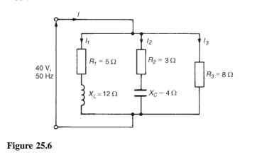
Impedance  $Z_1 = (5 + j12)\Omega$ ,  $Z_2 = (3 - j4)\Omega$  and  $Z_3 = 8 \Omega$ Supply current  $I = \frac{V}{Z_T} = VY_T$  where  $Z_T = \text{total}$  circuit impedance, and  $Y_T = \text{total}$  circuit admittance.
