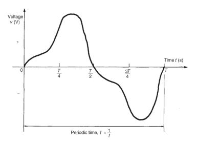
Figure 36.1 Typical complex periodic voltage waveform
