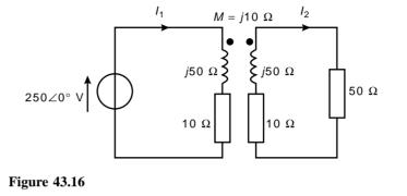
The position of the dots and the current directions correspond to Figure 43.15(a), and hence the signs of the M and L terms are opposite. Applying Kirchhoff's voltage law to the primary circuit gives:
