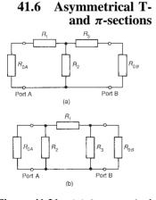
**Figure 41.21** (a) Asymmetrical *T*-pad section, (b) Asymmetrical  $\pi$ -section
