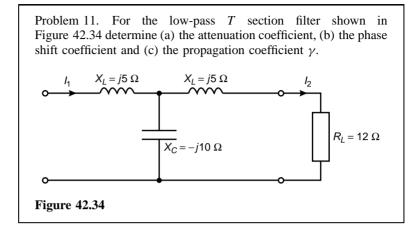
By current division in Figure 42.34,  $I_2 = \left(\frac{X_C}{X_C + X_L + R_L}\right) I_1$
