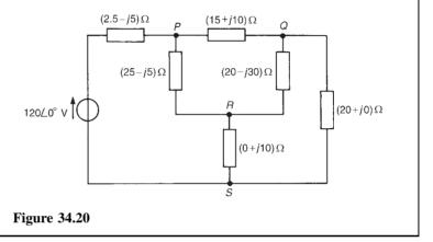
(a) The network may initially be simplified by transforming the delta PQR to its equivalent star connection as represented by impedances  $Z_1$ ,  $Z_2$  and  $Z_3$  in Figure 34.21. From equation (34.7),
