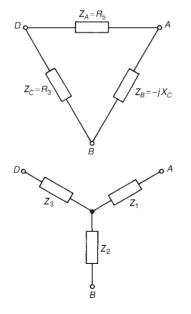
The network of Figure 34.16 is redrawn with the star replacing the delta as shown in Figure 34.18, and further simplified in Figure 34.19. (Note that impedance  $Z_1$  does not affect the balance of the bridge since it is in series with the detector.)
