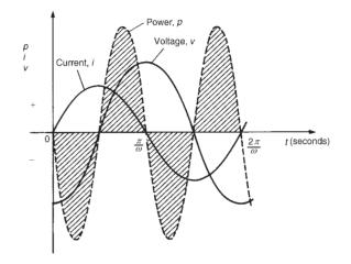
Figure 26.3 Power in a purely capacitive a.c. circuit
