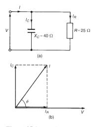
**Figure 25.1** (a) Circuit diagram, (b) Phasor diagram
