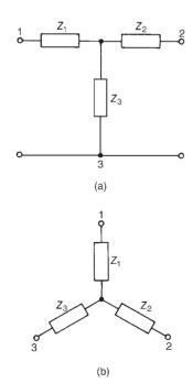
Figure 34.2 (a) T-connected network, (b) Star-connected network
