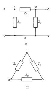
**Figure 34.1** (a)  $\pi$ -connected network, (b) Delta-connected network
