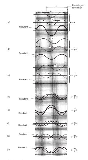
Figure 44.12 Voltage waveforms on an open-circuited transmission line
