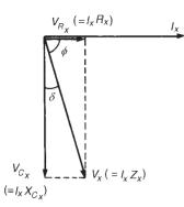
Figure 27.8 Phasor diagram for the unknown arm in the Schering bridge
