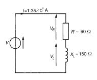
Problem 8. A circuit comprises a resistance of 90  $\Omega$  in series with an inductor of inductive reactance 150  $\Omega$ . If the supply current is  $1.35\angle 0^\circ$  A, determine (a) the supply voltage, (b) the voltage across the 90  $\Omega$  resistance, (c) the voltage across the inductance, and (d) the circuit phase angle. Draw the phasor diagram.
