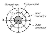
**Figure 40.11** *Electric field between two concentric cylinders*
