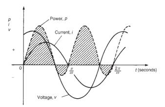
**Figure 26.4** *Power in a.c. circuit containing resistance and inductive reactance*
