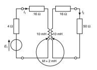
Problem 10. For the circuit shown in Figure 43.9, determine the value of the secondary current  $I_2$  if  $E_1 = 220^\circ$  volts and the frequency is  $\frac{10^3}{\pi}$  Hz.
