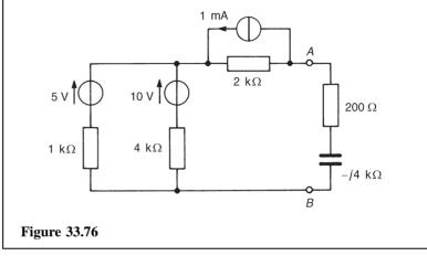
For the branch containing the 5 V source, converting to a Norton equivalent network gives  $I_{SC} = 5/1000 = 5$  mA and  $z = 1 \text{ k}\Omega$ . For the branch containing the 10 V source, converting to a Norton equivalent network gives  $I_{SC} = 10/4000 = 2.5$  mA and  $z = 4 \text{ k}\Omega$ . Thus the circuit of Figure 33.76 converts to that of Figure 33.77.
