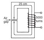
Problem 14. A section through a magnetic circuit of uniform cross-sectional area  $2 \text{ cm}^2$  is shown in Figure 7.5. The cast steel core has a mean length of 25 cm. The air gap is 1 mm wide and the coil has 5000 turns. The B-H curve for cast steel is shown on page 78. Determine the current in the coil to produce a flux density of 0.80 T in the air gap, assuming that all the flux passes through both parts of the magnetic circuit.
