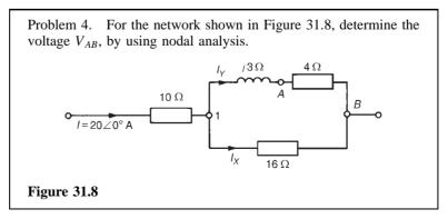
Figure 31.8 contains two principal nodes (at 1 and B) and thus only one nodal equation is required. B is taken as the reference node and the equation for node 1 is obtained as follows. Applying Kirchhoff's current law to node 1 gives:
