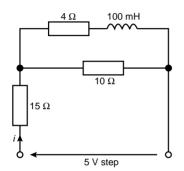
Problem 35. In the series-parallel network shown in Figure 45.24, a 5 V step voltage is applied at the input terminals. Determine an expression to show how current i varies with time.
