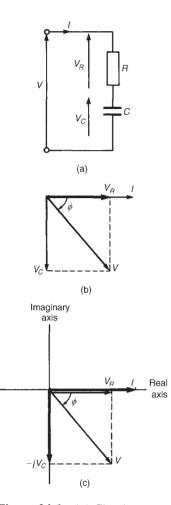
**Figure 24.6** (a) Circuit diagram (b) Phasor diagram (c) Argand diagram
