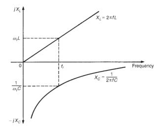
**Figure 28.3** Variation of  $X_L$  and  $X_C$  with frequency
