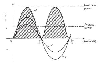
Figure 26.1 The waveforms of v, i and p
