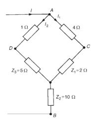
The network of Figure 34.12 may thus be redrawn as shown in Figure 34.14. The 4  $\Omega$  and 2  $\Omega$  resistances are in series with each other, as are the 1  $\Omega$  and 5  $\Omega$  resistors. Hence the equivalent network is as shown in Figure 34.15. The total equivalent resistance across terminals A and B is given by
