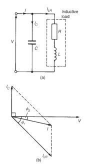
**Figure 26.11** (a) Circuit diagram (b) Phasor diagram
