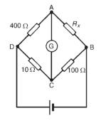
Figure 10.21 shows a Wheatstone bridge circuit which compares an unknown resistance  $R_x$  with others of known values, i.e.  $R_1$  and  $R_2$ , which have fixed values, and  $R_3$ , which is variable.  $R_3$  is varied until zero deflection is obtained on the galvanometer *G*. No current then flows through the meter,  $V_A = V_B$ , and the bridge is said to be 'balanced'.
