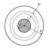
Figure 40.18 Cross-section of a concentric cable
