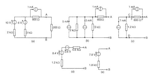
For the branch containing the 10 V source, converting to a Norton equivalent network gives
