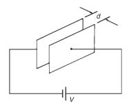
Figure 6.3 shows two parallel conducting plates separated from each other by air. They are connected to opposite terminals of a battery of voltage V volts.
