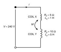
Problem 6. Two mutually coupled coils X and Y are connected in series to a 240 V d.c. supply. Coil X has a resistance of 5  $\Omega$ and an inductance of 1 H. Coil Y has a resistance of 10  $\Omega$  and an inductance of 5 H. At a certain instant after the circuit is connected, the current is 8 A and increasing at a rate of 15 A/s. Determine (a) the mutual inductance between the coils and (b) the coefficient of coupling.
