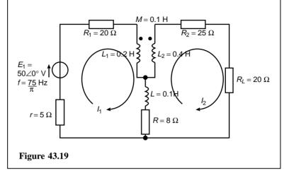
(a) The left hand mesh equation in Figure 43.19 is:
