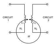
Mutual inductance is said to exist between two circuits when a changing current in one induces, by electromagnetic induction, an e.m.f. in the other. An ideal equivalent circuit of a mutual inductor is shown in Figure 43.1.
