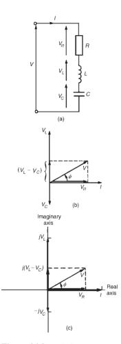
**Figure 24.8** (a) Circuit diagram (b) Phasor diagram (c) Argand diagram
