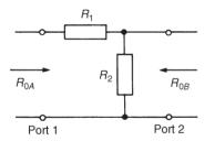
**Figure 41.31** *L-section attenuator pad*
