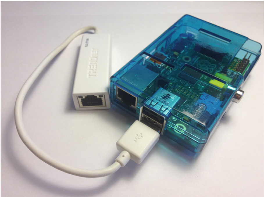
Fig. 3. Implementation of the SBF using a Raspberry Pi microcomputer. Two USB ports are used for exchanging commands with the PLC (with a network adapter) and the other SBF, using an USB radio frequency module.
