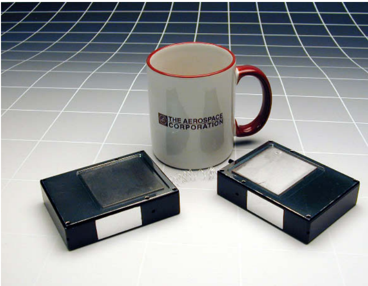
FIGURE 6-1-1 DARPA/Aerospace Corp. picosatellites. Photograph reprinted with the permission of the Aerospace Corporation.
