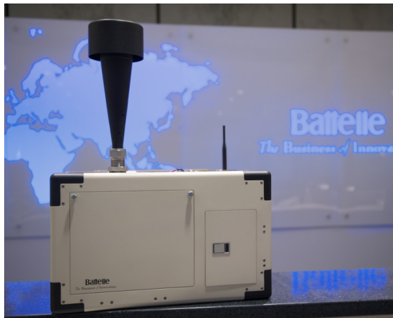
FIGURE H-7 Battelle's Resource Effective Bio-Identification System (REBS) provides collector, detector, and identifier functions within a single, portable system.
