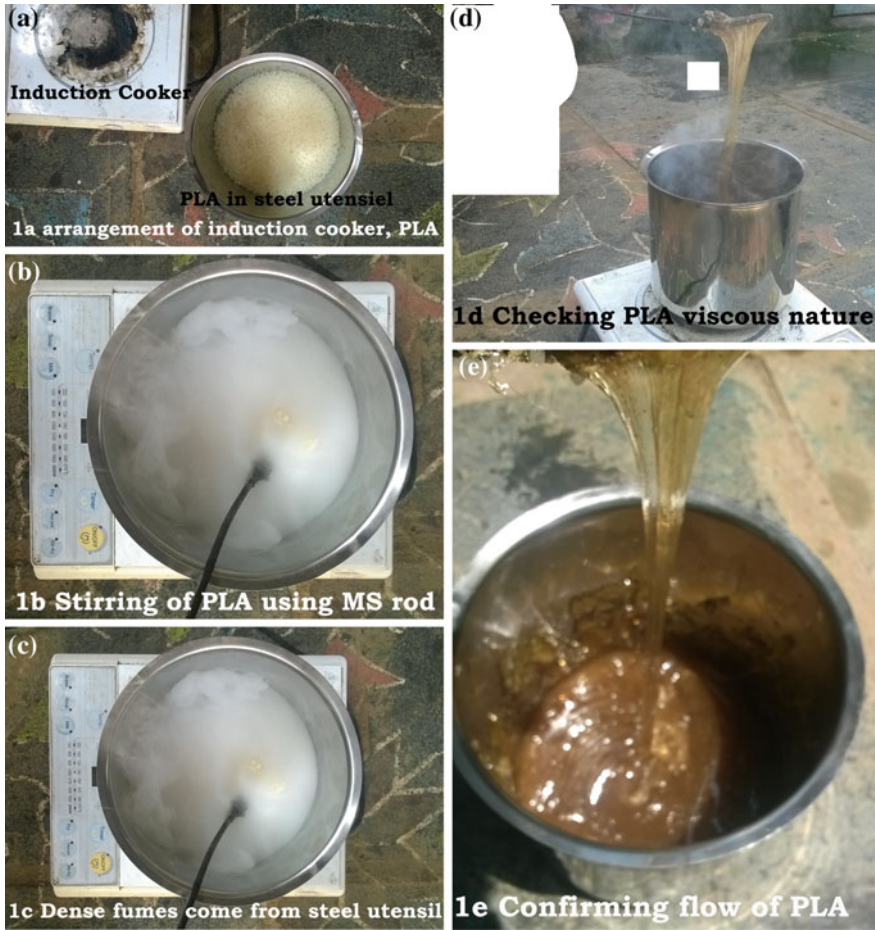
Fig. 1 Steps involved in lamina PLA, PLA-SBP composite lamina preparation and cutting of specimens
