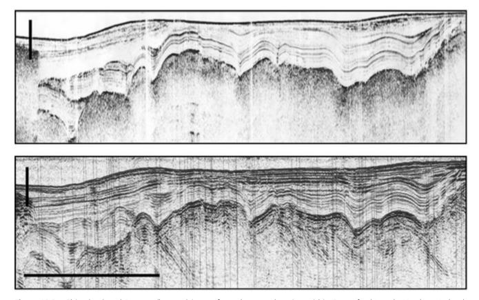
**Figure 13.3** Chirp (top) and Boomer (bottom) image from the same location within Strangford Lough, Northern Ireland, showing the detailed layering within the upper, fine-grained sediments in the Chirp profile and the penetration through stiff glacial sediments into the basal bedrock from the Boomer section. Data acquired using a GeoAcoustics Chirp and Boomer system. Vertical scale bar represents c.15 m (49 ft). (Courtesy of the National Oceanography Centre/University of Southampton)
