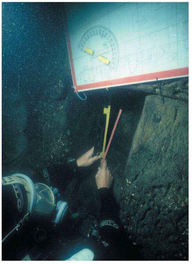
Plate 14.3 The clinometer in use measuring the angles of timbers on the Duart Point wreck. (Photo: Colin Martin)
