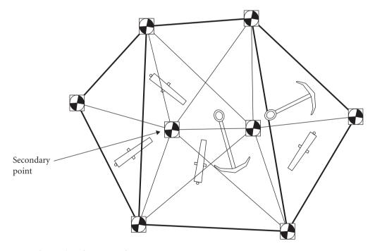
Figure 14.16 Secondary points (3-D survey)
