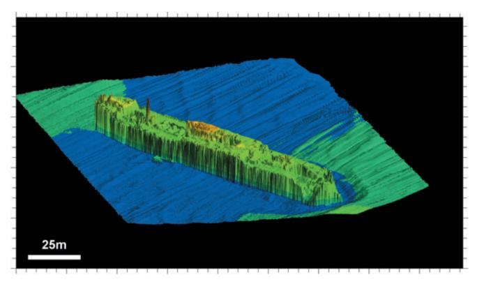
**Plate 13.3** Multibeam sonar image of the SS *Storaa* (1943) demonstrating the disadvantage of using a rendered surface, which can give wrecks a false slab-sided appearance. (Courtesy of ADUS, University of St Andrews)
