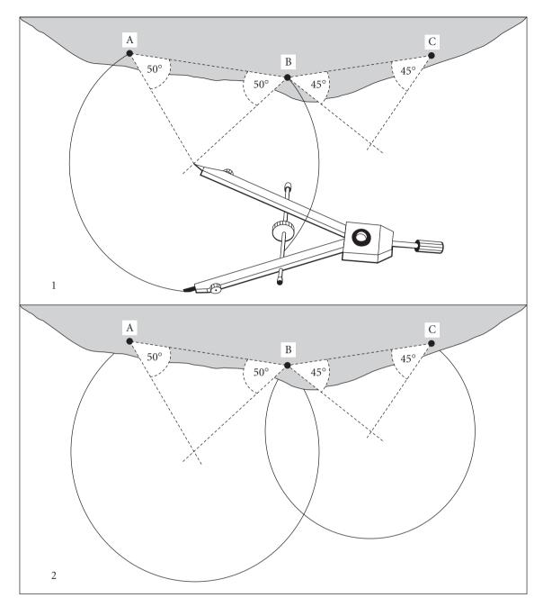
Figure 11.6 Sextant angles can be plotted geometrically from baselines between charted features. (Based on original artwork by Ben Ferrari)
