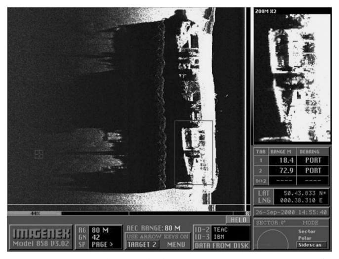
**Figure 13.2** Sidescan sonar image of the SS *Storaa* (1943) showing shadow detail complementing the backscatter information from the wreck. (Courtesy of ADUS, University of St Andrews)
