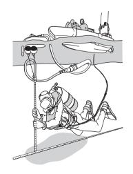
**Figure 15.3** Air or water probes can be used to explore a site but are potentially destructive. In this example, measurements (distance along tape and depth of probe) are being relayed to the boat via diver-to-surface communications. (Based on original artwork by Ben Ferrari)
