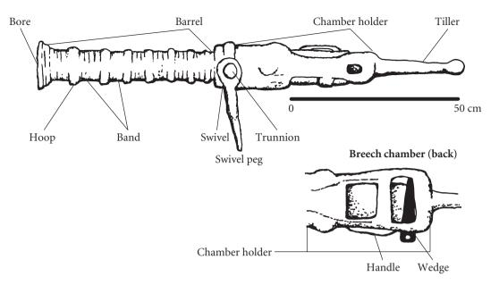
**Figure A2.3** Breech-loading swivel-gun: terminology – a corresponding recording form is available on the NAS website. (Based on original artwork by Ben Ferrari)
