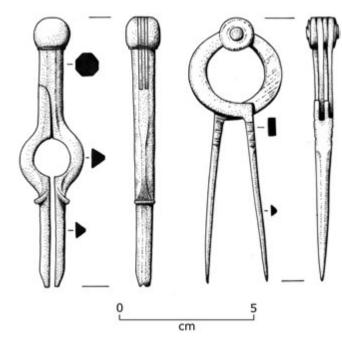
**Figure 18.13** Two pairs of brass dividers from the *Dart-mouth* (1690), of different designs. Front and side views of each instrument are shown, with sections where appropriate. Stippling is used to convey details and the matted surface of the metal. (Colin Martin)
