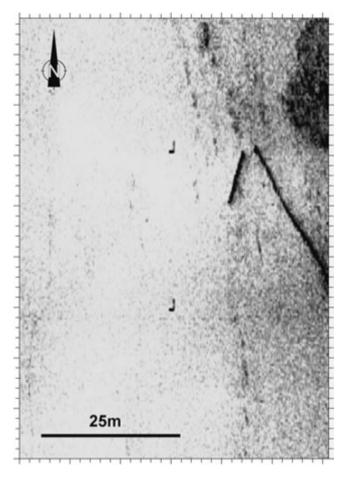
**Figure 13.1** 500 kHz sidescan sonar image of a v-shaped fish-trap from the River Barrow, County Wexford, Ireland. Data acquired using an EdgeTech Model 272-TD acquisition system. (Courtesy of the Centre for Maritime Archaeology, University of Ulster, Coleraine)
