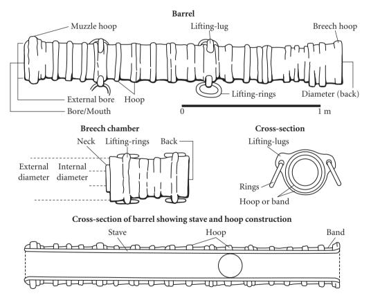
**Figure A2.2** Wrought-iron breech-loading tube gun: terminology – a corresponding recording form is available on the NAS website. (Based on original artwork by Ben Ferrari)
