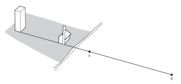
**Figure 11.9** Accuracy of transits: a position fix at A will be more accurate than at B. (Based on original artwork by Ben Ferrari)
