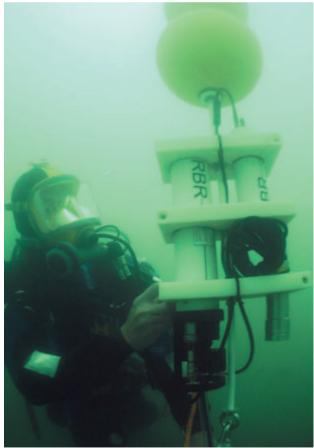
**Plate 17.2** Monitoring of the underwater environment (both sediments and water column) on the *Mary Rose* (1545) wreck using an RBR data-logger. This records temperature, pressure (depth), conductivity, salinity, pH, dissolved oxygen and turbidity. (Photo: Mary Rose Trust)
