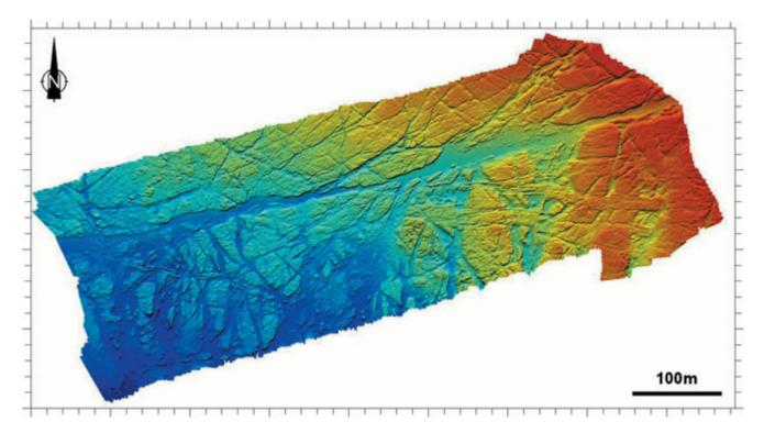
**Plate 13.2** Surface rendered multibeam sonar image of rock gullies off Moor Sand, UK, containing bronze-age and seventeenth-century material. The 700 m (2275 ft) long area runs WSW to ENE and is 260 m (845 ft) at its widest. (Courtesy of ADUS, University of St Andrews)
