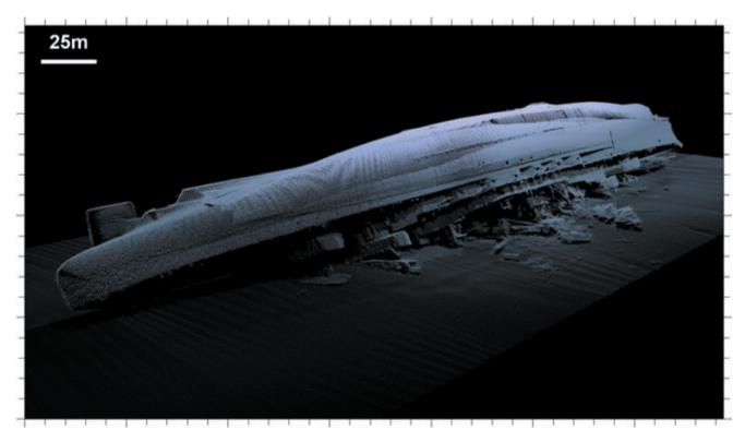
**Plate 13.1** High-definition multibeam sonar point-cloud image of the 203 m (660 ft) long wreck of HMS *Royal Oak* (1939) in Scapa Flow, Orkney. (Courtesy of ADUS and the Department of Salvage and Marine, Ministry of Defence)
