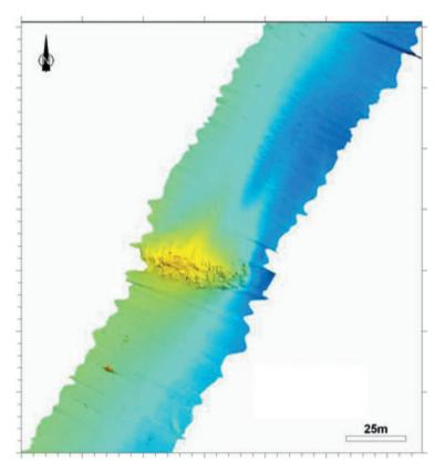
**Plate 13.7** Multibeam image from a single pass in 2002 showing the sea-bed around the wreck of the *Stirling Castle* (1703). The wreck mound is 46 m (150 ft) long. (Courtesy ADUS, University of St Andrews).
