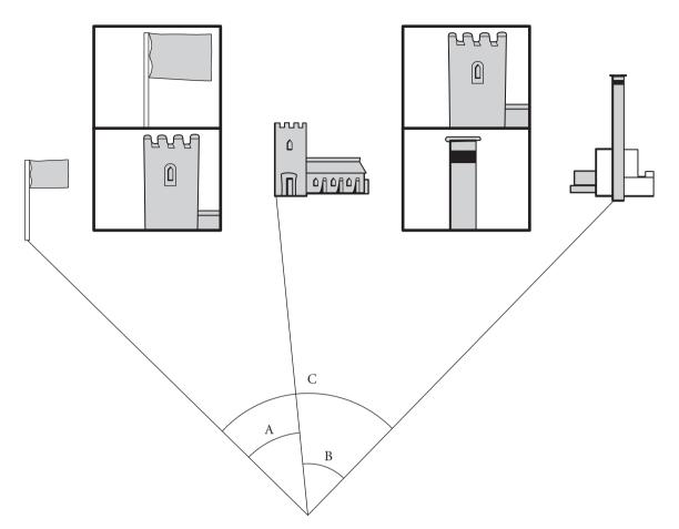
**Figure 11.4** Taking horizontal sextant angles. Angle A is measured between left-hand side of the flagpole and the left-hand side of the church tower by lining them up in the split-viewfinder. Angle B is measured between the left-hand side of the church tower and the left-hand side of the chimney. Angle C, measured between the flag pole and the left-hand side of the chimney, should equal angle A plus angle B. (Based on original artwork by Ben Ferrari)
