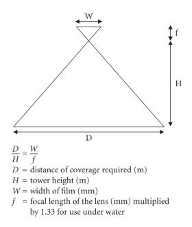
**Figure 10.8** Photomosaics: formula to calculate lens focal length and camera height necessary to give the required coverage. (After Green, 2004:171)
