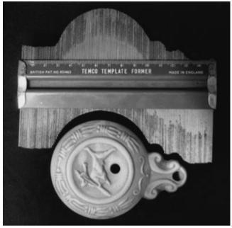
**Figure 18.10** Profile gauges can provide a quick way of checking the shape of an object but they can easily damage delicate surfaces and should only be used on robust items. Their use is not generally recommended in recording small finds (for which better techniques are available), but they can be useful for recording features such as the mouldings on guns. (Photo: Colin Martin)
