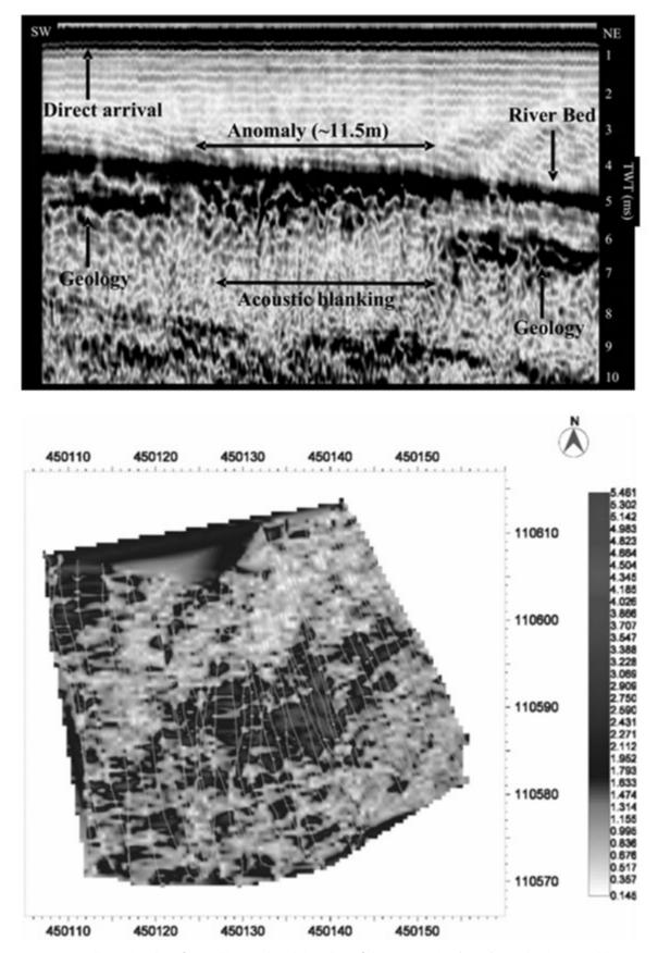
**Figure 13.4** A two-dimensional profile and interpolated timeslice of the *Grace Dieu* (1439) wreck, River Hamble, Hampshire, UK. Data acquired using a 3-D Chirp sub-bottom profiling system, developed by the National Oceanography Centre and GeoAcoustics Ltd (UK). (Courtesy of the National Oceanography Centre/University of Southampton)
