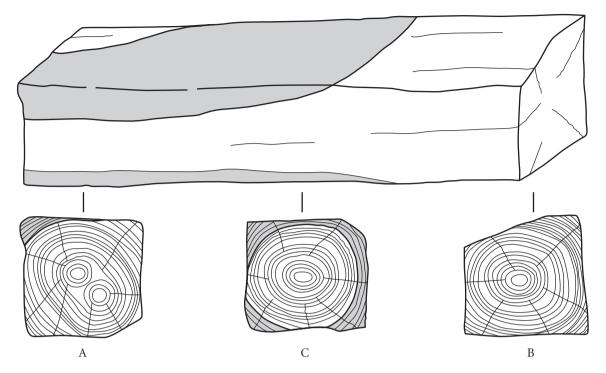
**Figure 15.4** Optimum place for tree-ring sampling: A) branching is distorting the ring pattern, B) no sapwood is present, C) there is undistorted ring growth and good sapwood survival. (Based on original artwork by Ben Ferrari; after Nayling, 1991:47)
