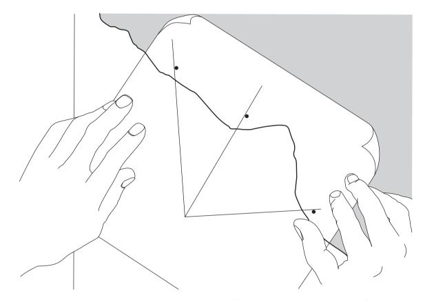
**Figure 11.5** Sextant angles can be scribed on plastic drafting film to within about 20 minutes of arc (one-third of a degree). This can be sufficiently precise to plot a position on a large-scale chart. (Based on original artwork by Ben Ferrari)
