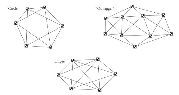
Figure 14.15 Good control-point network shapes (3-D survey)
