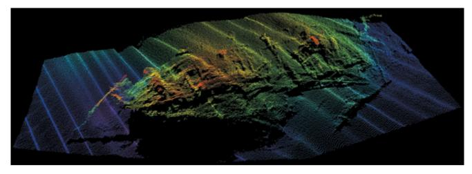
**Plate 13.9** Multibeam image of a nineteenth-century wooden sailing ship on the Goodwin Sands at the entrance to the Strait of Dover. The end of the bowsprit now rests on the sea-bed but when surveyed 12 weeks earlier, it was in its operational position. (Courtesy of ADUS and the RASSE Project, University of St Andrews)
