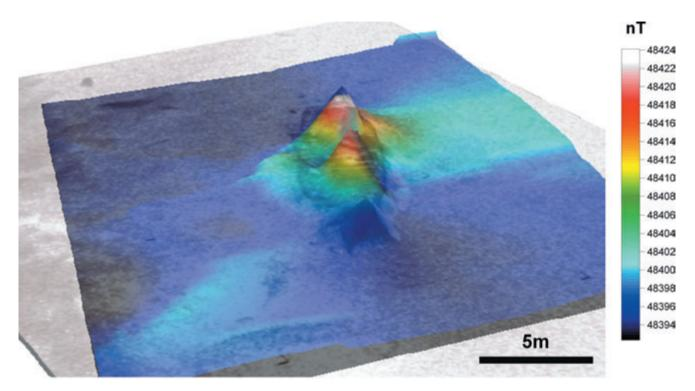
**Plate 13.11** Three-dimensional plot of magnetic data acquired from the *La Surveillante* (1797) wreck-site, Bantry Bay, County Cork, Ireland. (Courtesy of the Centre for Maritime Archaeology, University of Ulster, Coleraine and the Applied Geophysics Unit, National University of Ireland, Galway)
