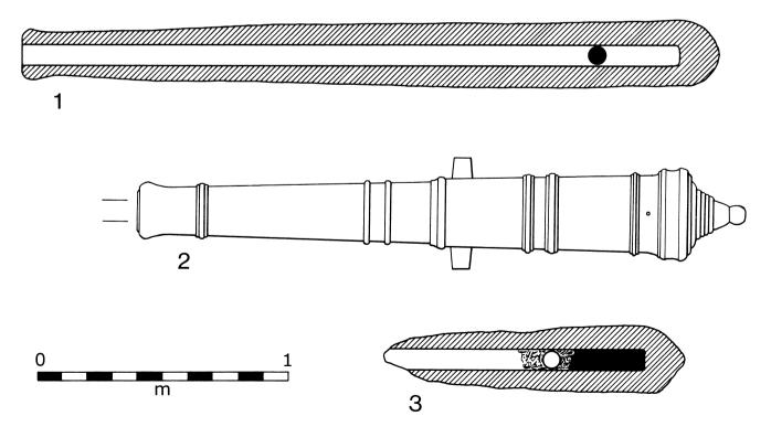
**Figure A2.10** Plain iron guns from the Armada wreck *El Gran Grifon* (1588): 1) shows the sectioned shape of one gun within an abraded concretion deposit, with its iron roundshot still in place; 2) is the profile of a complete gun (a side or frontal view would be needed to show the set of the trunnions); while 3) is an abraded fragment within which the roundshot, wadding and powder charge are preserved. (Colin Martin)
