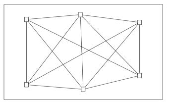
Figure 14.14 Measuring between quads (3-D survey)
