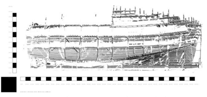
**Figure 18.17** An orthographic view of the shaded 3-D laser-scan data of the *Mary Rose* (1545) hull. As the scanner operates in a 'line-of-sight' manner, the timbers near the top have been obscured from the scanning viewpoint near the ground. (Copyright Archaeoptics Ltd; reproduced courtesy of the Mary Rose Trust).
