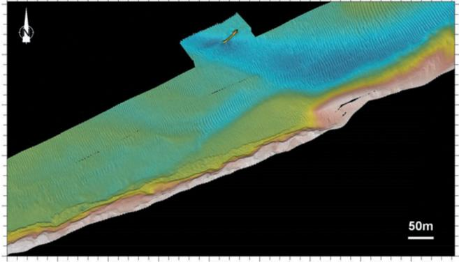
**Plate 13.4** Multibeam image of a prehistoric land surface at the base of the 8 m (28 ft) high underwater Bouldner Cliff in the Solent, UK. The wreck of the 44 m (143 ft) long dredger *Margaret Smith* (1978) is included for scale. (Courtesy of ADUS, University of St Andrews)
