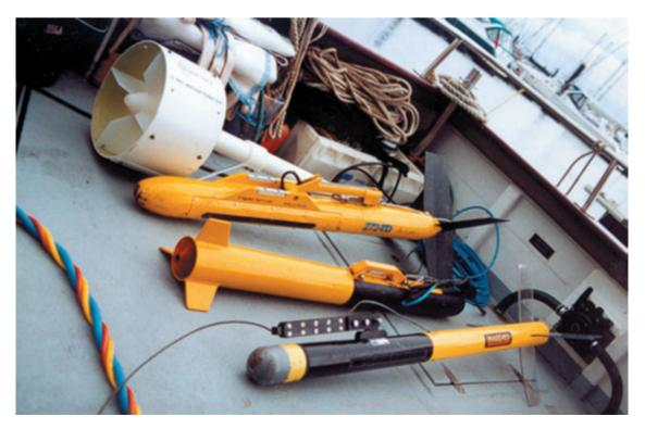
**Plate 13.12** Top to bottom: a Geometrics G-881 caesium magnetometer (white tow-fish), an EdgeTech 272–TD side-scan, a GeoAcoustics side-scan and an Imagenex 885 side-scan sonar. (Photo: Rory Quinn)
