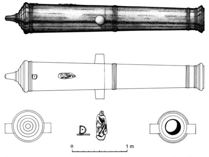
**Figure A2.11** A drawing properly set out for publication of a piece of ordnance – a cannon perrier (designed for stone shot) from a Spanish Armada wreck off Streedagh Strand, Ireland. (Doug McElvogue)
