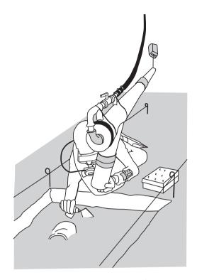
**Figure 15.11** Water-dredge operation. (Based on original artwork by Ben Ferrari)
