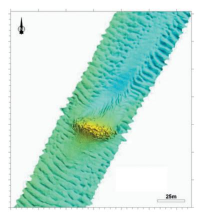
**Plate 13.8** Multibeam image from a single pass in 2005 showing the sea-bed around the wreck of the *Stirling Castle* (1703). Well-defined sand waves have developed around the wreck mound in the 3 years since the previous survey shown in plate 13.7. (Courtesy of ADUS and the RASSE Project, University of St Andrews)
