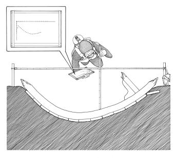
**Figure 14.4** Recording the profile of a wreck using vertical offsets from a horizontal datum. (Drawing by Graham Scott)
