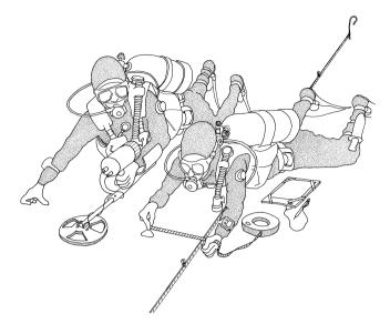
**Figure 12.3** The offset method can be used to record the position of features in relation to jackstays and ground-lines. In this example a hand-held metal-detector is being used to locate metallic features. (Drawing by Graham Scott)
