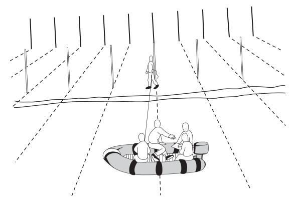
**Figure 11.10** Temporary transits formed by setting up paired ranging rods along a shore baseline. When collecting data close inshore, or on inland waters, additional locational control can be provided by a tape measure or a distance line. (Based on original artwork by Ben Ferrari.)
