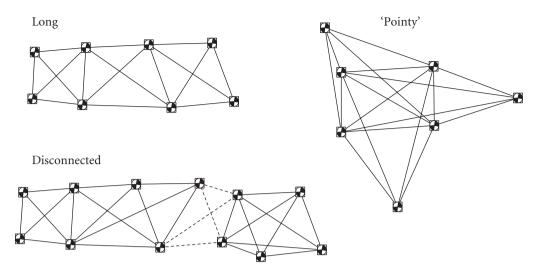
Figure 14.17 Poor control-point network shapes (3-D survey).
