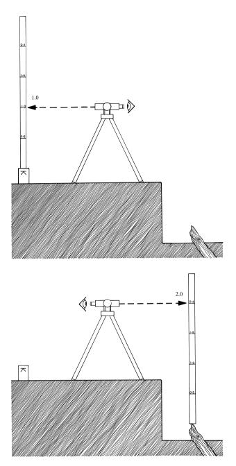
**Figure 14.7** The principle of levelling to establish relative heights/depths. For example, if the benchmark is at 6 m: top image shows the level is 6 + 1 = 7 m above chart datum; bottom image shows the level is 2 m above timber; therefore, top of protruding timber is 7 - 2 = 5 m above chart datum. (Drawing by Graham Scott)
