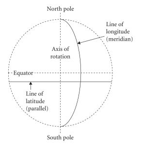
Figure 11.1 The earth, showing latitude, longitude and equator
