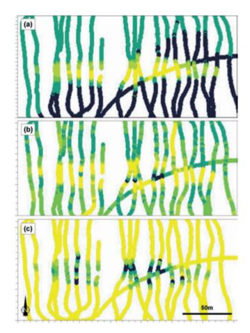
**Plate 13.10** Ground-discrimination data collected from a single-beam echo-sounder showing (a) bathymetry, (b) hardness and (c) roughness of the wreck of the 178 m (580 ft) long *Markgraff* (1919) in Scapa Flow. (Courtesy of Mark Lawrence, ADUS, University of St Andrews)
