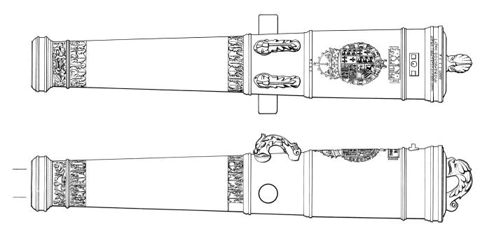
**Figure A2.5** Plan and side view of a decorated cast-bronze gun from the Spanish Armada (1588) wreck *La Trinidad Valencera*. (Colin Martin)
