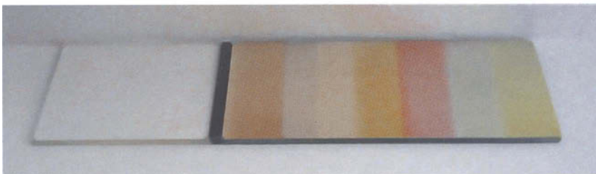
Figure 5.26. Fluorescence amplification in a Ag-cluster-layer – SnNx-interlayer system (steps from 0 700 nm) , photo (fewer steps than scan above).
