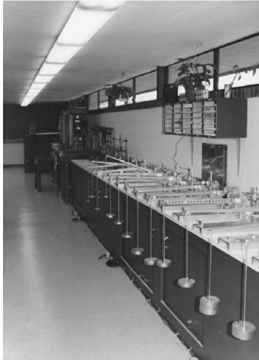
FIGURE 5.2 Modified Consolidation Test.
