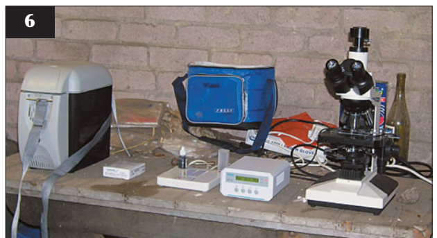
6 The field laboratory shown here includes a warming box and heated stage to keep semen at body temperature during examination for motility.
