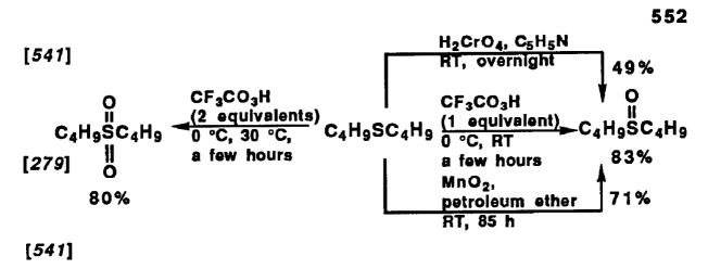
Organic peroxy acids, especially at low temperatures, oxidize sulfides to sulfoxides [163, 324], whereas tetrabutylammonium persulfate [209] at room temperature and hydrogen peroxide at higher temperatures yield sulfones [163, 324]. However, hydrogen peroxide in acetic anhydride at room temperature yields sulfoxides [166]. Under these conditions, double bonds resist epoxidation [163, 166, 324] (equation 553).
