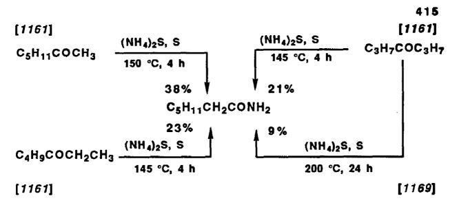
The amides and thioamides obtained by the Willgerodt-Kindler reaction are, sometimes without isolation, converted into acids by refluxing with 15–20% sodium or potassium hydroxide or converted into esters by refluxing for 3 h with alcohols in the presence of gaseous hydrogen chloride [501].
