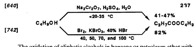
The oxidation of aliphatic alcohols in benzene or petroleum ether with tert-butyl chromate at 1–2 °C for 6 h leads to mixtures of aldehydes, acids, and their esters. Butanol gives 30% of butanal, 27% of butyric acid, and 36% of butyl butyrate [677]. Also, electrolysis of aliphatic alcohols on platinum or carbon electrodes in aqueous potassium iodide at room temperature results in 80–83% yields of the corresponding esters [121].
