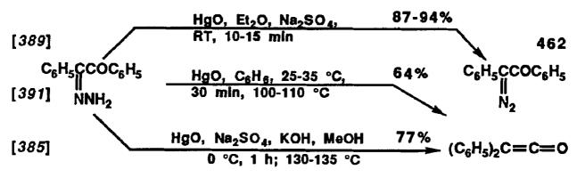
Dihydrazones of  $\alpha$ -diketones, when treated with mercuric oxide at higher temperatures, yield *acetylenes* [393, 394, 395, 396]. Diphenylacetylene is obtained by refluxing benzil dihydrazone with mercuric oxide [396] in benzene or by refluxing benzil monohydrazone with mercurous trifluoroacetate in ether for 2 h (yield 43%) [405]. The oxidation of dihydrazones
