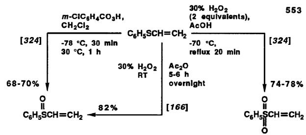
The oxidation reagents used most frequently for the conversion of sulfides into sulfoxides and sulfones are hydrogen peroxide, peroxy acids, and periodates. Periodates usually do not oxidize sulfoxides to sulfones [770 771, 772, 776, 778]. In addition, many other, even rather exotic, oxidants have been used especially for chemoselective oxidations of sulfides containing functional groups vulnerable to attack by peroxy compounds, such as double bonds and carbonyl groups.
