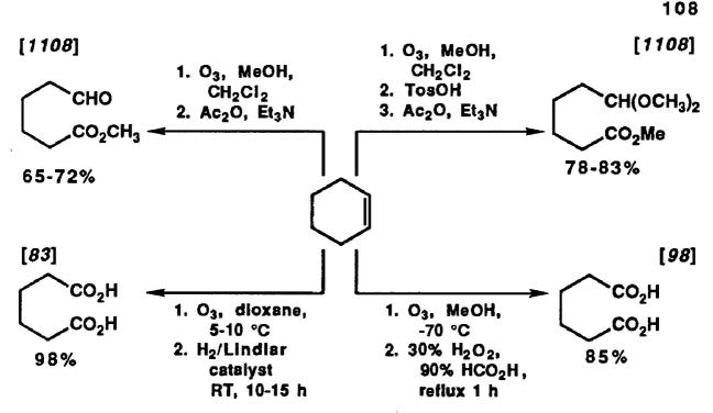
The oxidative decomposition of ozonides is further accomplished by their treatment with **hydrogen peroxide** [97] in the presence of formic acid [98, 99] or acetic acid [102, 103] or with silver oxide and nitric acid [77] (equations 109-112).
