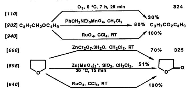
\*Support on silica gel is essential for such work, because zinc permanganate is a potentially dangerous reagent [898].
