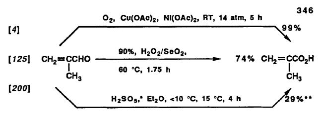
$^*\mathrm{H}_2\mathrm{SO}_5$  is prepared either by adding ammonium persuifate to 85% sulfuric acid below 15 °C, or by adding 90% hydrogen peroxide to concentrated sulfuric acid below 15 °C, and keeping the mixture for 2 h at room temperature.
