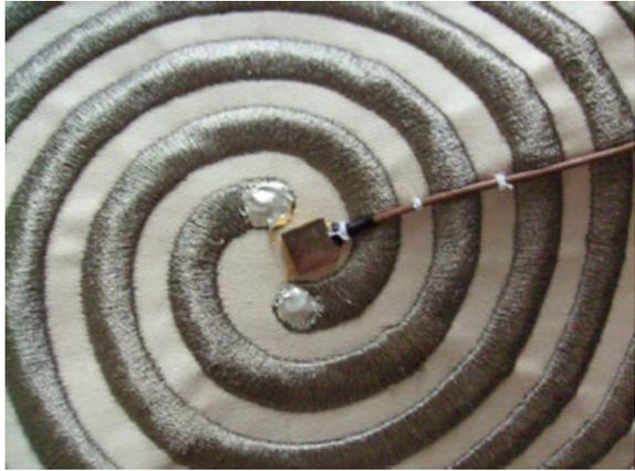
**Fig. 6** Copper coated fabric bow tie antenna
