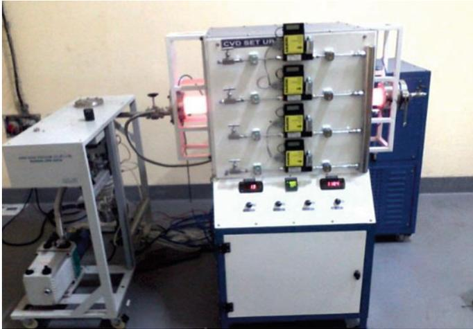
**Fig. 1** Image of thermal CVD set up
