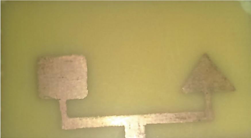
Fig. 5 1 × 2 hybrid patch array antenna
