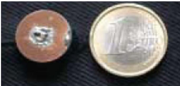
Fig. 3 Textile layer small size button antenna with (left)
