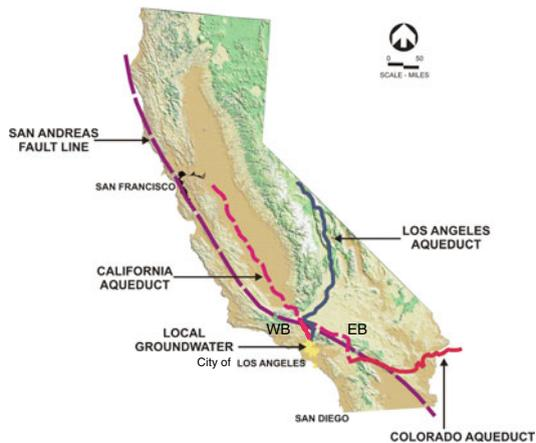
**Fig. 3.7** California map showing Los Angeles megacity water supply sources from the Los Angeles Aqueduct, Colorado River Aqueduct, and California Aqueduct. EB and WB are the California Aqueduct East and West Branches, respectively. The San Andreas Fault is shown to pass nearly the entire length of the state. The City of Los Angeles is shown matching that area presented in Fig. 3.5a; the Los Angeles megacity area is presented in Figs. 3.2 and 3.5b
