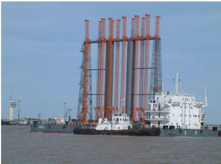
**Fig. 7.10** Offshore PVD installation barge (after Yan et al., 2009)
