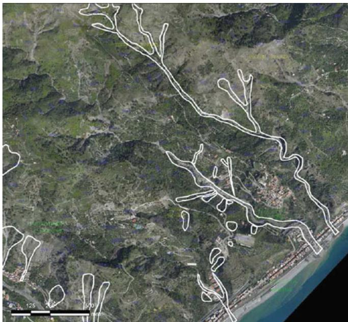
**Fig. 10.7** Debris flow originated by the Saponarà, Racinazzi and Divieto streams at Scaletta
