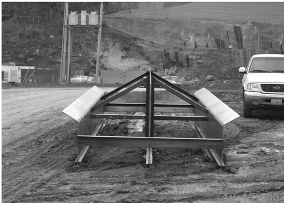
Figure 9.27 (a) Typical spreader box and screed (adapted from Charlton and Crane, 1980), (b) Spreader box from the rear and (c) Double spreader box (FEMA, 2011).
