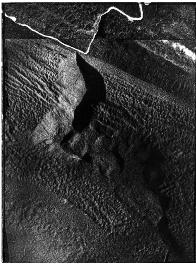
Figure 3.34 Air photo showing the scar of an old landslide in folded limestone, near the Mubi River, Papua New Guinea.
