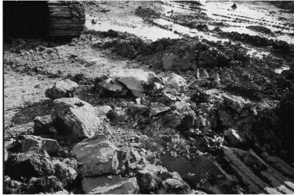
Figure 6.31 Fissures in pieces of weathered volcanic tuff. The fissures are induced by desiccation when the ground surface was exposed above sea level. Largest pieces are about 450 mm across.
