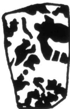
Fig. 1.2. Electrographic print of a nickel ore. The black parts represent the originally red spots of nickel dimethylglyoxime complex that have been formed where nickel ions were released into the reagent paper by oxidation of the nickel mineral 15
