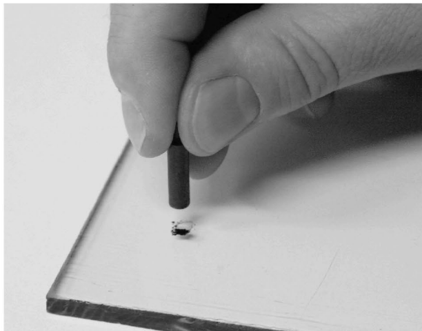
Fig. 3.2. Transfer of microparticles from a glass plate onto the surface of a paraffin impregnated graphite electrode (PIGE)
