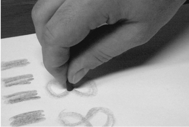
Fig. 3.3. Cleaning the surface of a PIGE by interrupted polishing on paper
