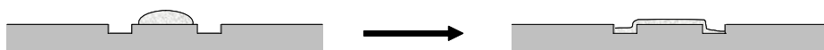
Fig. 1. Schematic view of the spread of the liquid on a structured substrate /2/
