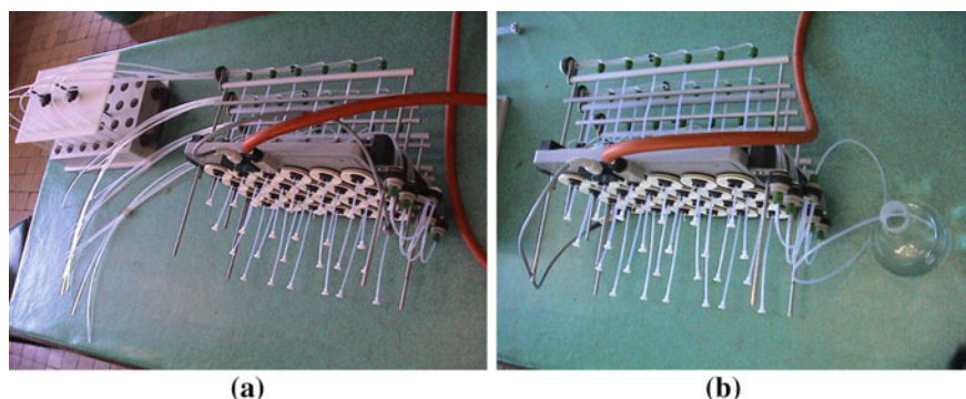
Fig. 5.5 Attachment for SynCore apparatus for parallel filtration of 24 suspensions: a for filtration (24 plastic tubings are attached to the left part of the attachment for forcing over the mother liquors) and b for washing (a bottle with a washing liquid is attached to the right part of the attachment)
