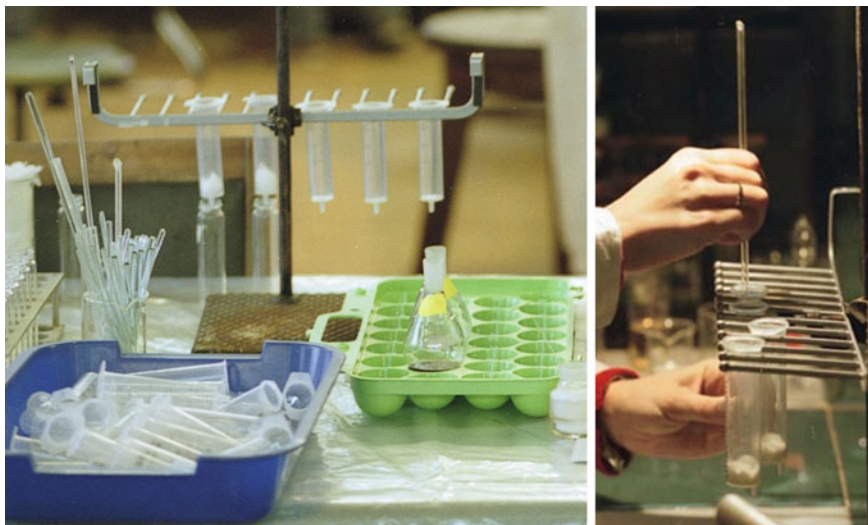
Fig. 4.1 Space-saving fastening of syringe columns in a manifold
