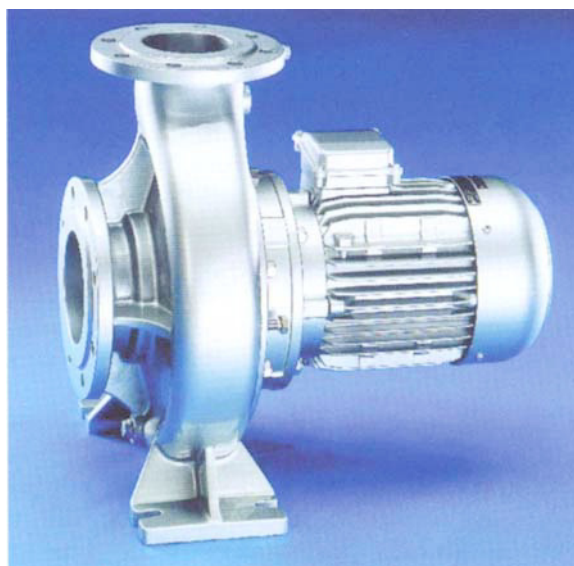
Figure 7.8. Circulating pump for solar loop, cast iron housing, chrome nickel steel shaft, cast iron or gunmetal impeller. Manufacturer: Herborner, Herborn
