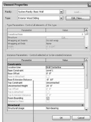
FIGURE 12.23 Modifying the wall layers
