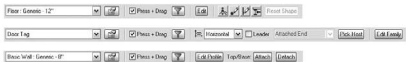
FIGURE 3.1 The tool set offered by the Options bar depends on the type of element you've selected.
