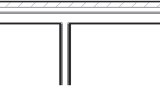
Figure 4.9 A stud wall joining to a brick wall in plan
