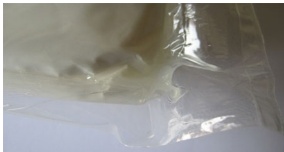
Fig. 1.11 Leakage of whey from inner packaging (parchment) to the area between packaging materials
