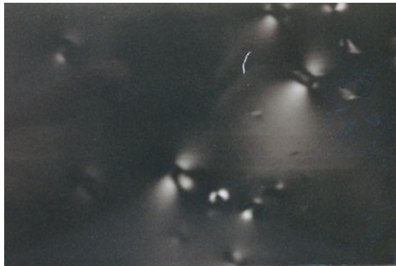
Fig. 1.10 PA/PE laminates after 14 days of contact with lactic acid
