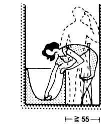
⑫ Minimum space between bath and wall
