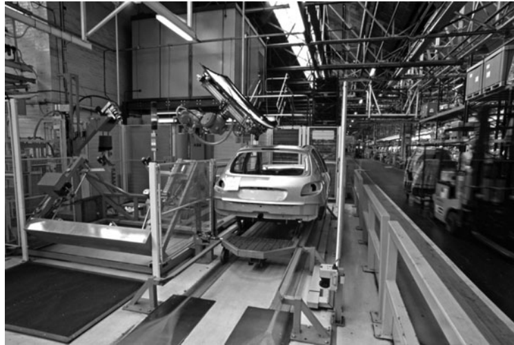
Peugeot assembly line. In this assembly line, each workstation is designed to perform a specific process. Thus, the car is constructed as it moves down the line and ultimately emerges as a finished product.
