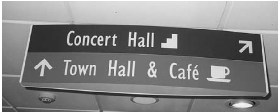
Figure 4.58 Good use of text, contrast, symbols and directional arrows – and ideally sized, bearing in mind the distance from which it will be viewed.
