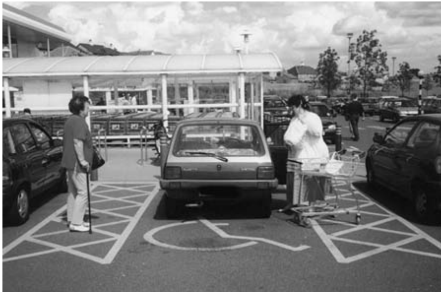
Figure 4.2 Parking bay with adequate room for both side and rear exit and entry to allow easy use. Although the rear exit and entry area is not marked, it can clearly be achieved without encroaching into the vehicle route.
