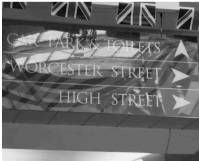
Figure 4.55 The incorrect use of surface finish can completely negate the effectiveness of a sign, especially in certain lighting situations. Non-reflective surface finishes for signs are essential.
