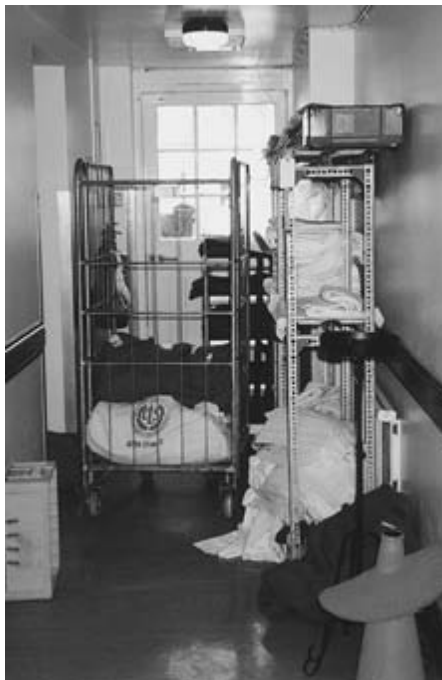
Figure 2.1 Obstructions such as these should be identified as problems associated with working practices. Assessing if it is a space problem or a staff training issue should be part of any access audit.
