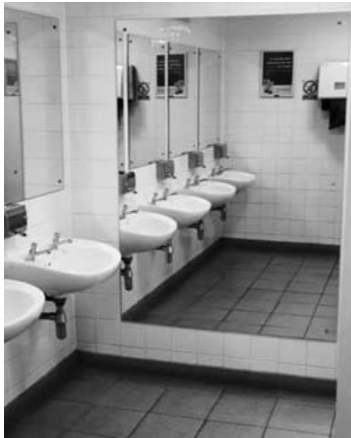
Figure 4.48 The use of large floor-to-ceiling mirrors can cause confusion and should be avoided.
