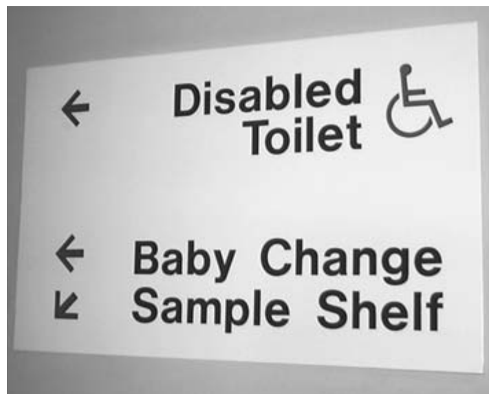
Figure 4.57 Good clear signage, though the word Disabled is unnecessary. Toilet or WC accompanied by the symbol is sufficient.
