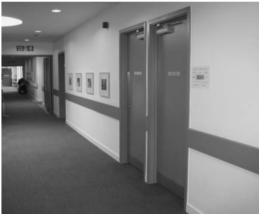
Figure 4.54 Visual contrast can be used to assist orientation and identify features.
