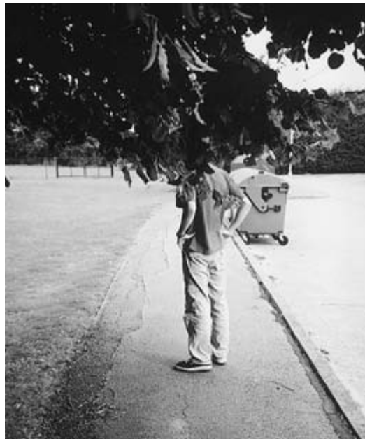
Figure 4.12 Projections into the walking zone can be very dangerous for all people, but especially people with visual impairments. Projections should be avoided, or at least properly protected, at all times.
