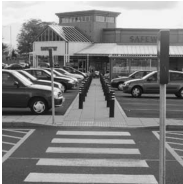
Figure 4.3 Good clear signage, correct drainage, and firm non-slip surfaces are essential. Routes between parking areas should be clear and well defined; bollards can prevent encroachment.
