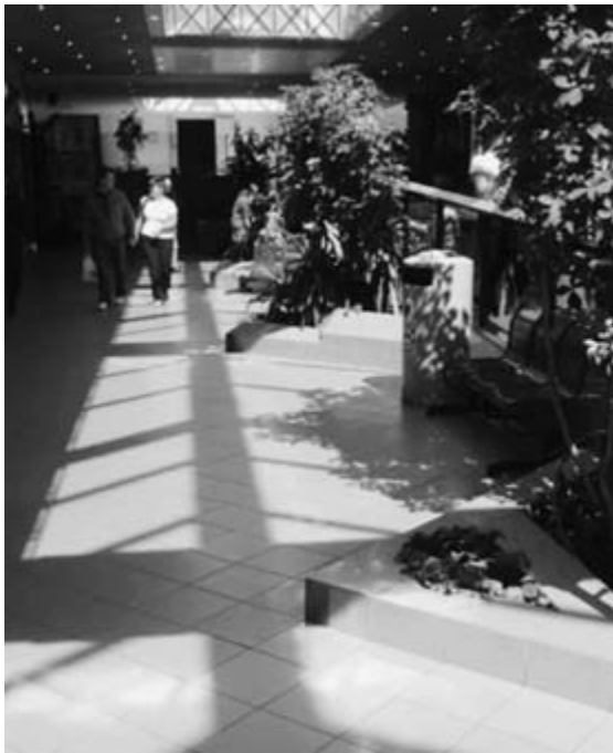
Figure 4.61 Strong shadows can cause confusion and make navigation difficult.
