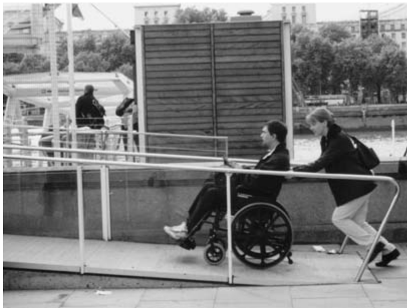
Figure 4.16 A ramp with a gradient of 1 in 12 may be too steep for people to use easily and conveniently.
