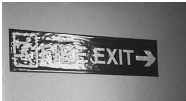
Figure 4.64 Fire exit signs should be located where they are clearly visible and care taken to ensure lighting does not cause reflections that obscure the information.
