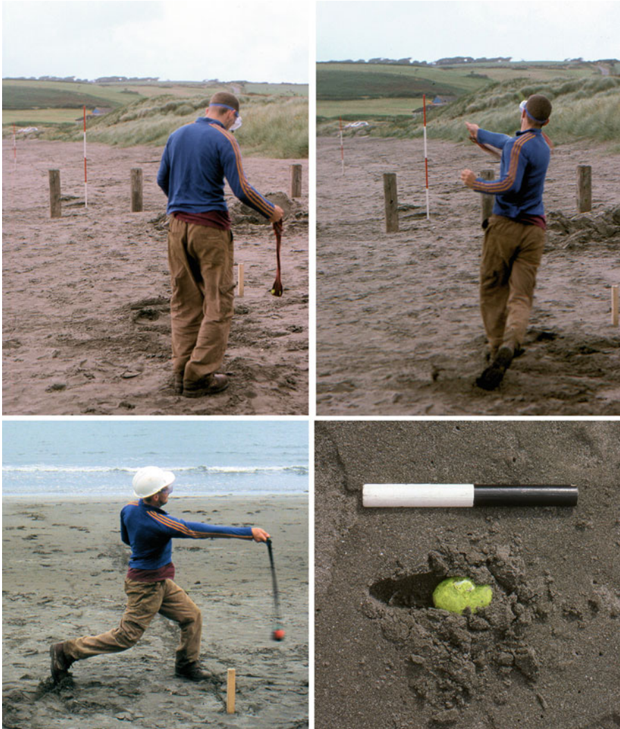
Fig. 15.6 Sling experiments. Top left and right: rear views of sling action. Bottom left: side view of sling action. Bottom right: impact of sling shot in sand
