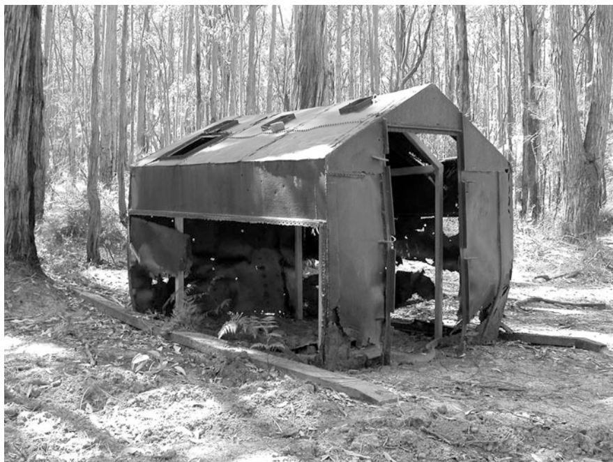
Fig. 8.7 Portable charcoal kiln in the Gembrook Forest east of Melbourne (photo P. Davies)
