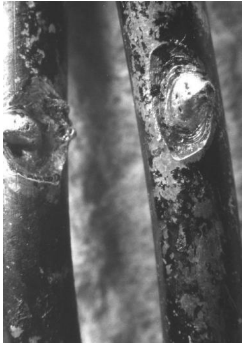
Figure 6.15 (See color insert.) Arced conductors.
