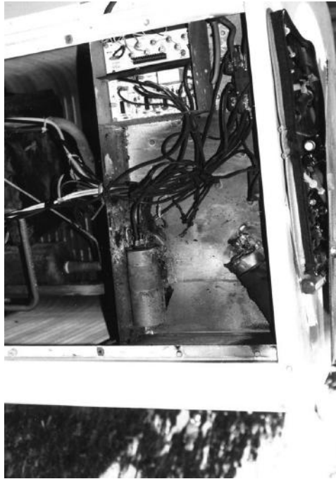
Figure 6.20 (See color insert.) Air conditioner fire.
