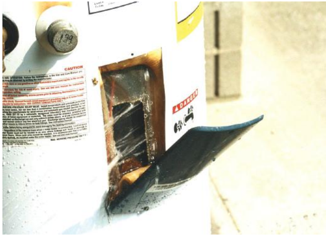
Figure 6.22 Failed water heater.
