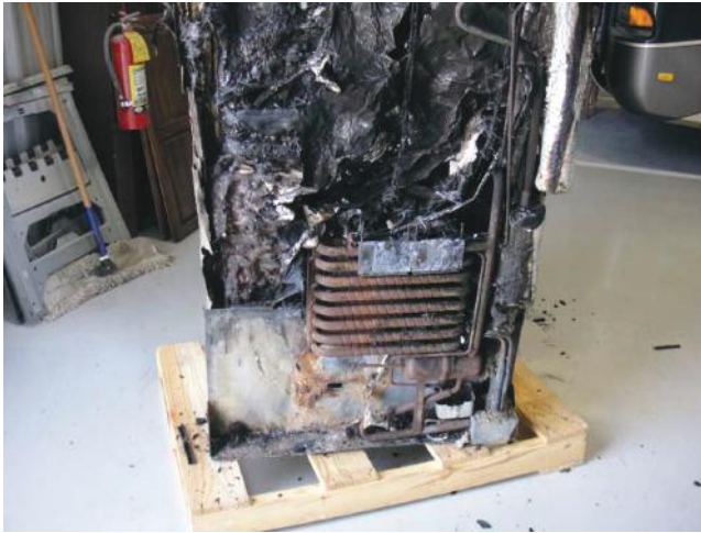
Figure 6.8 Absorption refrigerator fire.
