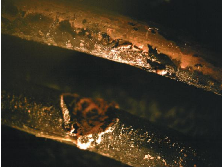
Figure 6.41 Arced solid conductors—saddle.
