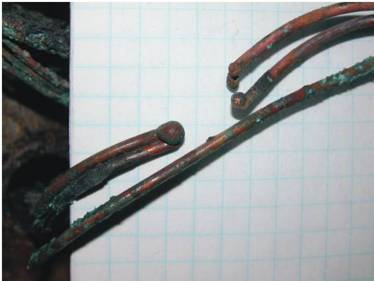
Figure 6.40 Arced solid conductors—beads.
