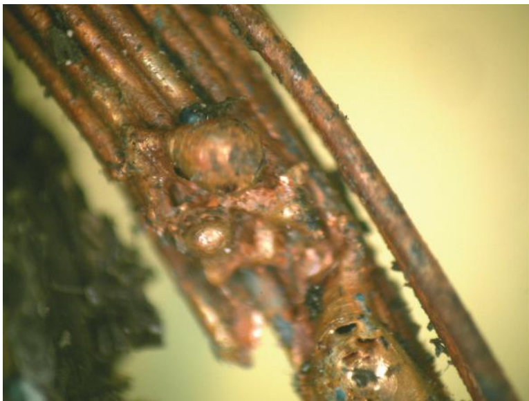
Figure 6.42 Arced stranded conductors—beads.
