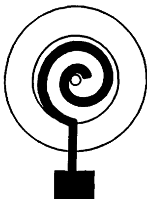
Figure 16.2 A microfabricated spiral shape sensing element used in microtitration application.
