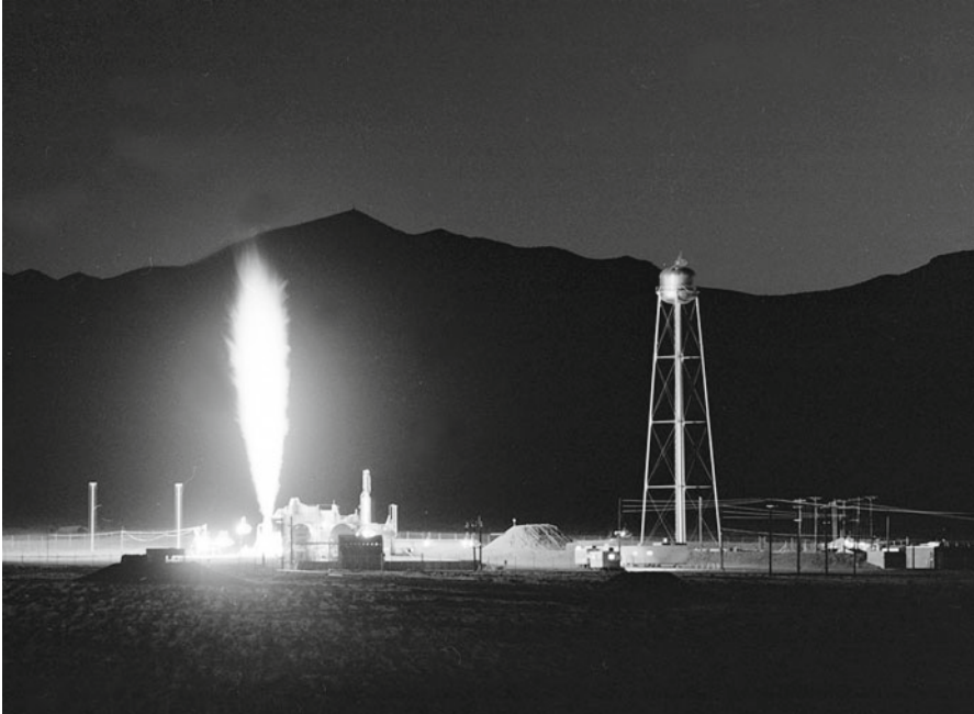
Fig. 5 Full power test of Kiwi B at Test Cell A (courtesy of Los Alamos National Laboratory)
