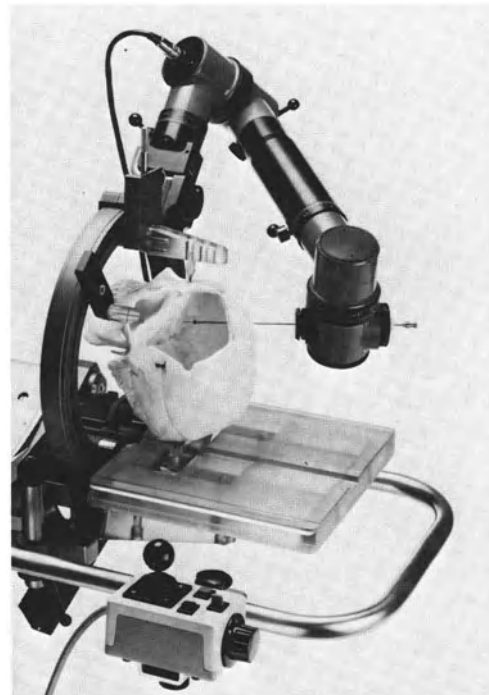
Fig. 1. Digitizing arm on halo-ring headholder. Bottom: control-panel
