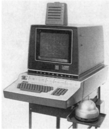
Fig. 1. Tektronix T-402 "Computer Graphics Terminal". To the right of keyboard, "Joystick", type 015-1075-00, controlling movable cross-hairs on screen
