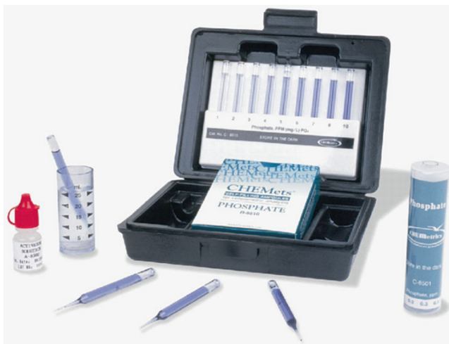
Fig. 4.4 Visual phosphate tests involve comparison of sample color with color intensity in a series of test vials. In this example, ten different vials of increasingly darker blue solutions are used. The darker the color, the higher the concentration of phosphate. This test kit is produced by the company CHEMetrics
