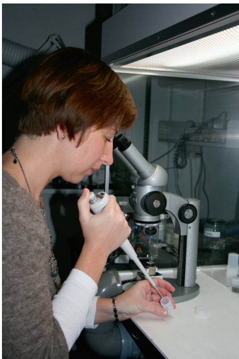
Fig. 4.20 Loading sample strontium solution on a filament for measurement in the thermal ionization mass spectrometer (TIMS)
