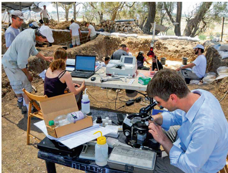
Fig. 1.1 Archaeological science in the field. Excavations in the background supply samples for a Fourier Transform Infrared Spectrometer, center, and microscopic identification, foreground. This project is at Tell es-Safi/Gath, an archaeological site in Israel occupied almost continuously from prehistoric to modern times. Photo courtesy of Kimmel Center for Archaeological Science, Weizmann Institute of Science, Israel
