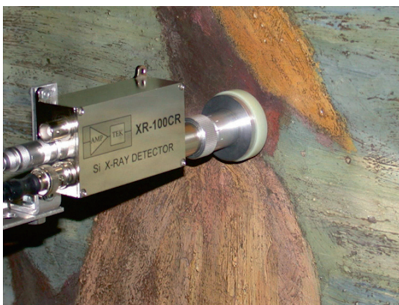
Fig. 3.10 Portable X-ray fluorescence instrument measuring composition of pigment in mural painting
